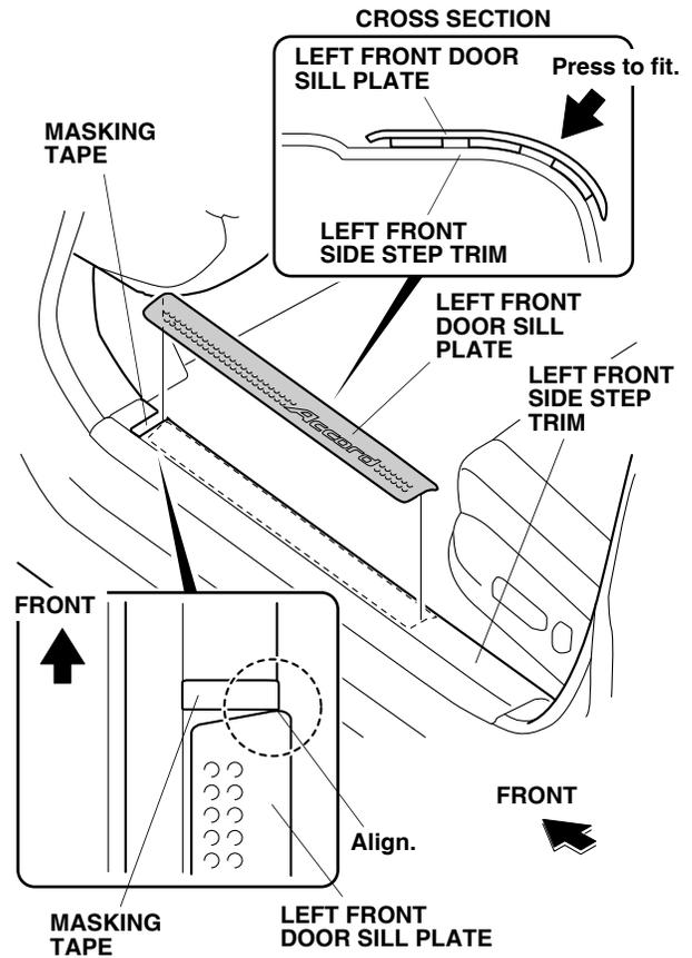
3. Using an alcohol swab, thoroughly clean the left front side step trim where the door sill trim will attach.
