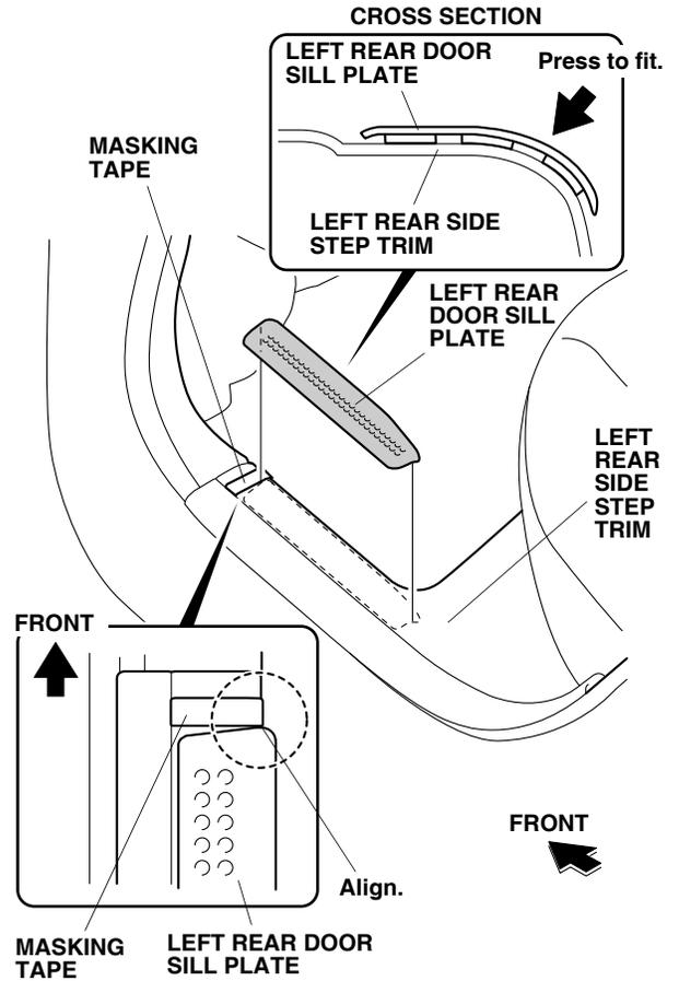
10. Using an alcohol swab, thoroughly clean the left rear side step where the rear door sill trim will attach.
