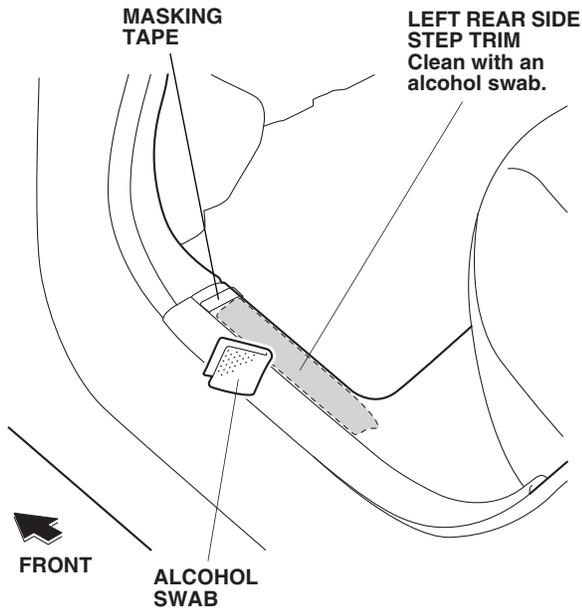
11. Attach pieces of masking tape to the ends of the adhesive backings as shown. Peel back the adhesive backings partway and temporarily attach them to the outer surface of the left rear door sill plate. Remove the remaining adhesive backings.
