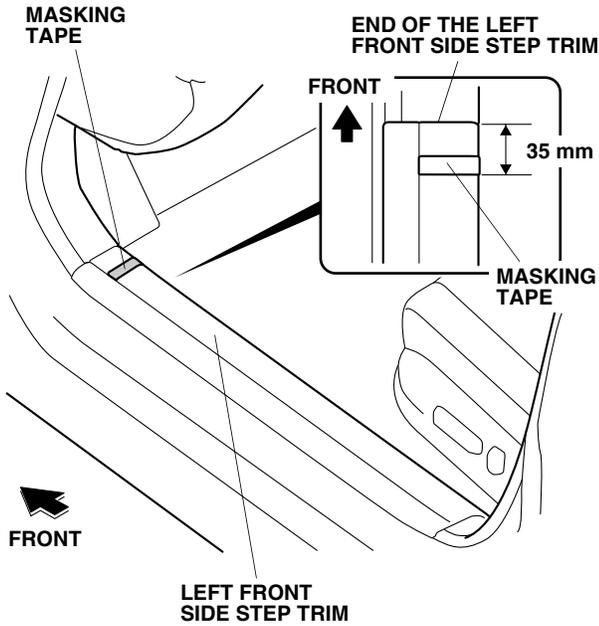
2. Align the front edge of the left front door sill plate to the masking tape attached in step 1, then press on the left front door sill plate to fit it to the left front side step trim as shown. Remove the door sill plate.
