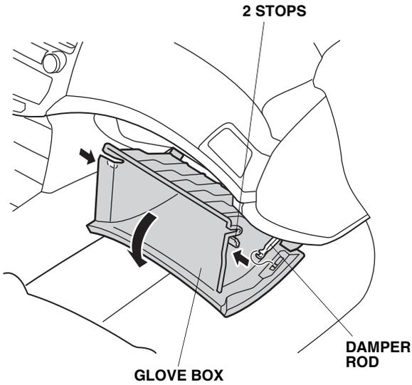
10. Remove the glove box (two screws).
