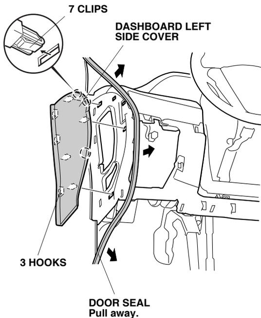
6. Remove the dashboard left side cover (seven clips and three hooks).
