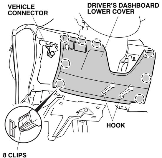
4. *V6 model only:* Remove the driver's dashboard under cover (three clips and one pin).
