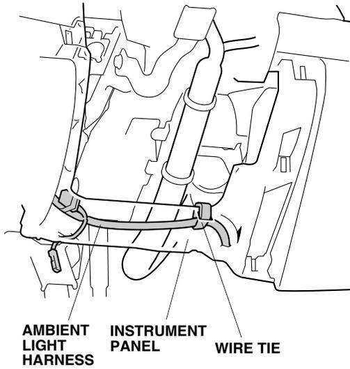
23. Attach a piece of steel wire to the ambient light harness with electrical tape, and route the ambient light harness through the center console from the foot well to the front passenger's foot well.
