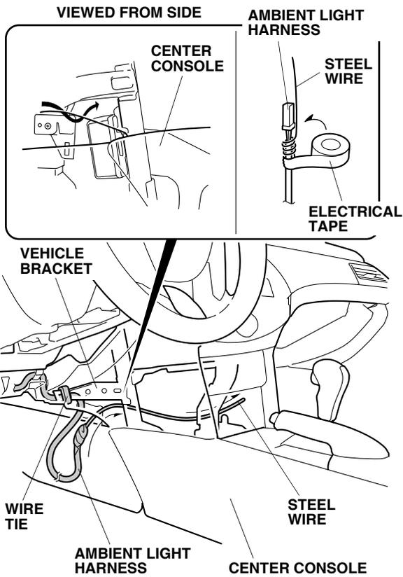
24. Secure the ambient light harness to the vehicle bracket with one wire tie.
