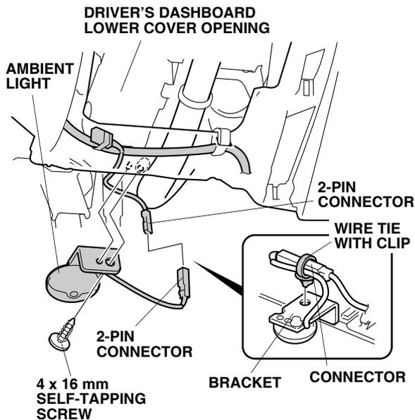
29. Install the ambient light to the passenger's side of the vehicle:
