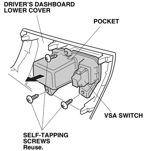
12. Release two retaining tabs and remove the VSA switch from the pocket. Set the pocket aside, it will not be reused.
