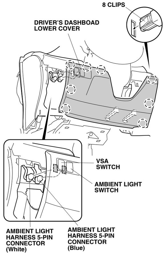
33. Check that all wire harnesses are routed properly and all connectors are plugged in.
