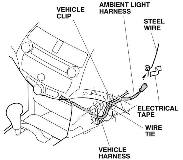
26. Route the ambient light harness. Secure the ambient light harness to the vehicle harness with one wire tie as shown.
