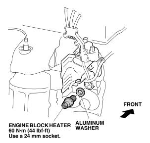
13. Plug the connector on the heater harness into the engine block heater. Route the heater harness as shown, and secure the two wire ties with clips (points A and B) to the vehicle bracket.
