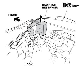
19. Route the heater harness as shown, and secure it to the vehicle harness with three black wire ties.
