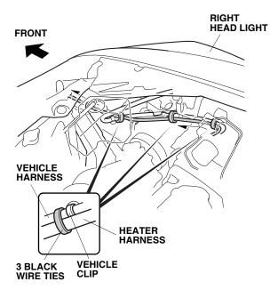
20. Route the heater harness as shown, and secure the wire tie with clip (point G) to the vehicle frame.
