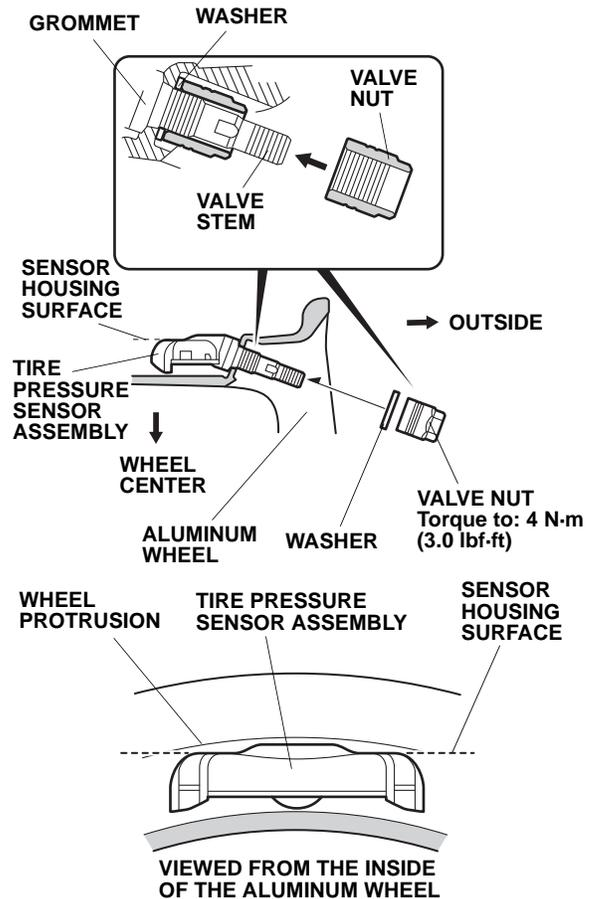
2. Install the tire pressure sensor assembly into the aluminum wheel. Install the washer, and finger-tighten the valve nut. Make sure the tire pressure sensor assembly is resting on the wheel, and does not protrude into the bead area of the wheel..
