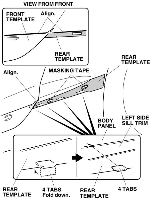
6. Align the rear template to the body panel and attach it with masking tape.
