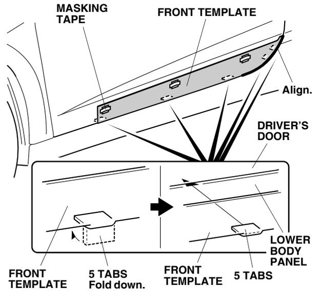
4. Align the front template to the driver's door and attach it with masking tape.
