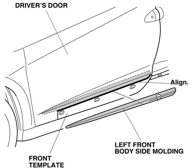
9. Peel back approximately 1½ to 2 inches of adhesive backing from each adhesive strip, and tape the ends to the front surface of the body side molding. Remove the end pieces of the adhesive backing.
