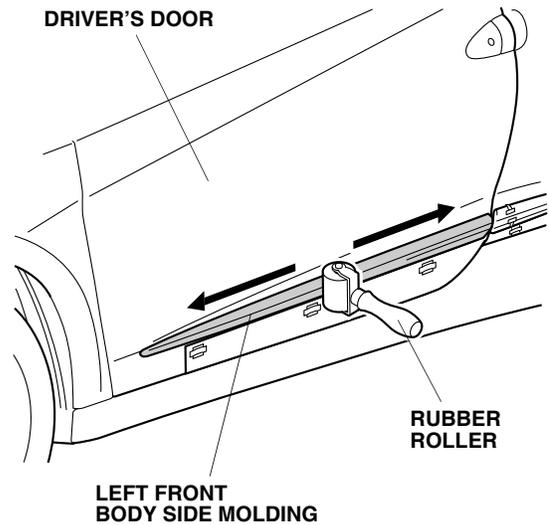
14. While pressing the body side molding firmly with the palm of your hand, remove the adhesive backings.
