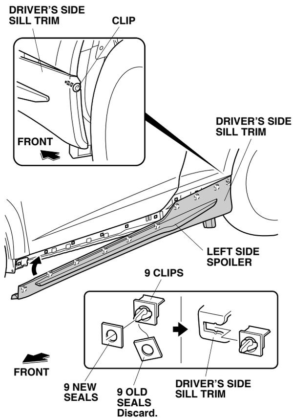
15. Install nine new seals onto the nine clips and install the nine clips onto the driver's side sill trim.
