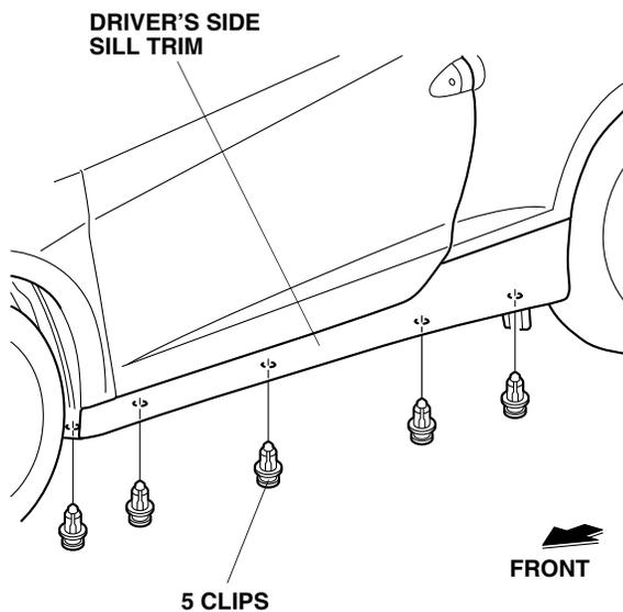
2. Remove the driver's side sill trim (nine clips). **NOTE:** Place the driver's side sill trim on a blanket after removal.
