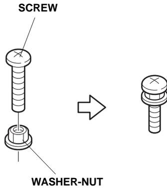
40. Using a Phillips screwdriver, securely tighten the screw into the clamp. Finger-tighten the washer-nut against the clamp. While holding the screw, tighten the washer-nut 90° clockwise with a 10 mm open end wrench.
