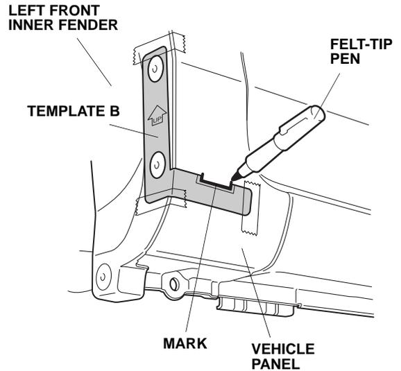
12. Carefully remove template B. Do not damage the template. It is also used for installing the right side spoiler.
