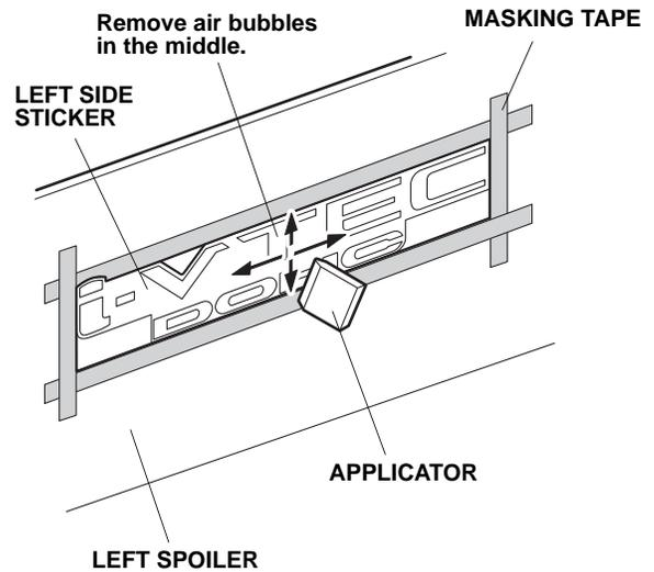
56. Spray the left side sticker again with 3M protective tape application solution. Remove the masking tape.
