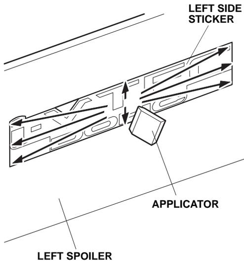
58. Use a shop towel to wipe the excess 3M protective tape application solution from the left side sticker. Allow the left side sticker to dry thoroughly.
