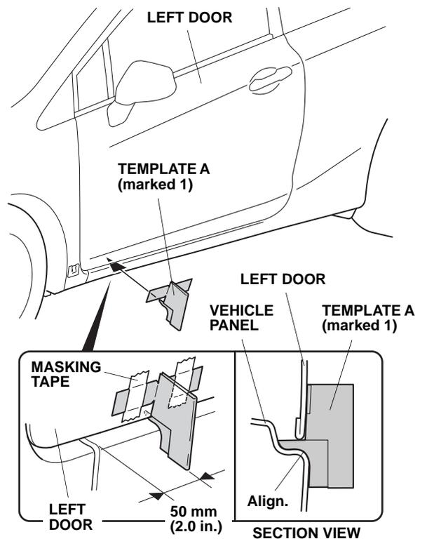
18. Place template A (marked 2) into position as shown. While aligning template A (marked 2) with the vehicle panel by lightly pushing down, attach template A (marked 2) to the left door using strips of masking tape. Make sure there is no gap between the template and the vehicle panel.
