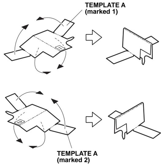
17. Place template A (marked 1) into position as shown. While aligning template A (marked 1) with the vehicle panel by lightly pushing down, attach template A (marked 1) to the left door with masking tape. Make sure there is no gap between the template and the vehicle panel.
