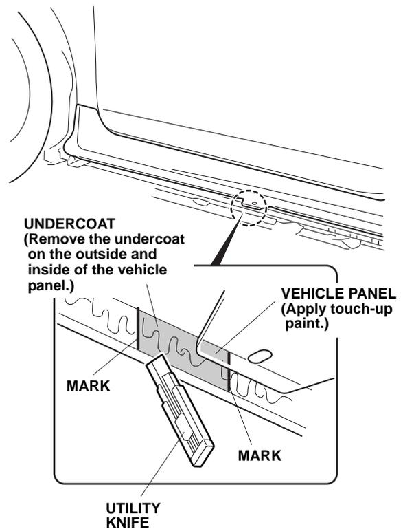
37. Apply touch-up paint to the area where the undercoat is removed, and allow it to dry thoroughly.
