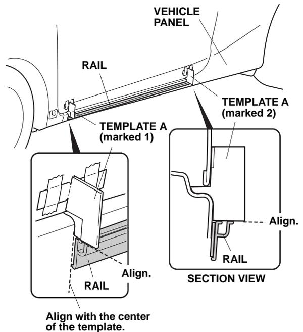
22. While making sure that the rail is aligned with the templates, carefully remove the adhesive backings.
