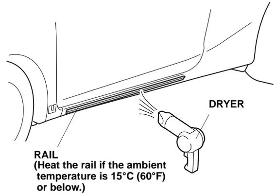
25. Using the palm of your hand, firmly press the rail against the vehicle panel.
