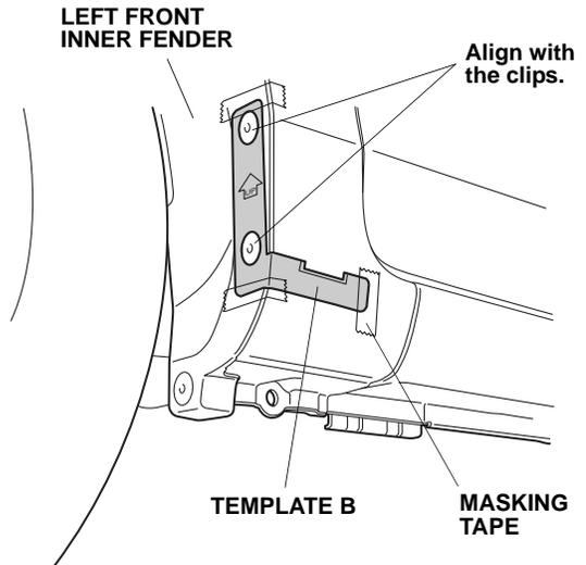
11. Using a felt-tip pen, mark the vehicle panel as shown.
