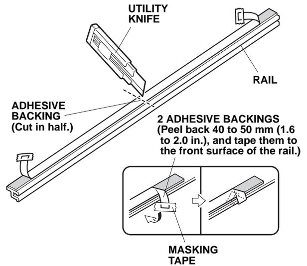
20. Peel back about 40 to 50 mm (1.6 to 2.0 in.) of adhesive backing from each adhesive strip, and tape the ends to the front surface of the rail.
