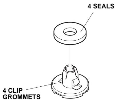
12. Install the clip grommets into the four holes in the trunk lid. Apply pressure to each clip grommet until you hear a click, and make sure it is installed securely.
