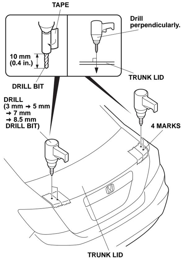
9. Remove the tape attached in step 2. Remove all burrs and metal shavings with a file, and apply touch-up paint to the edges of the holes.
