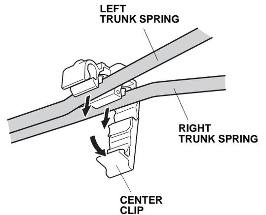
29. Wear heavy gloves to protect your hands. With an assistant holding the trunk lid open, use the trunk spring tool to remove the left trunk spring from the trunk lid right hinge. Pull the trunk spring tool slowly and carefully toward you.
