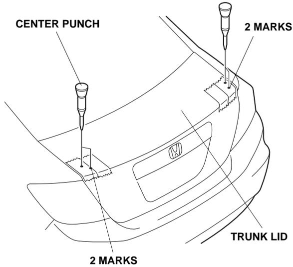
8. While wearing eye protection, drill four 8.5 mm holes through the marks. First drill with a 3 mm drill bit, then a 5 mm drill bit, then a 7 mm drill bit, and finish with an 8.5 mm drill bit. Drill perpendicularly to the trunk lid.
