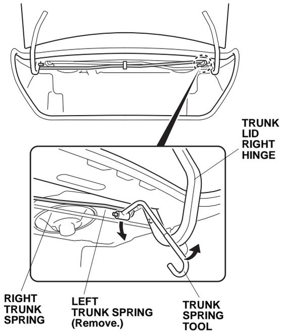
30. Install the new left trunk spring in the slot in the trunk lid left (driver's) hinge and to the right (passenger's side) hinge bracket. Set the trunk spring in the first notch (original position) of the hinge bracket.
