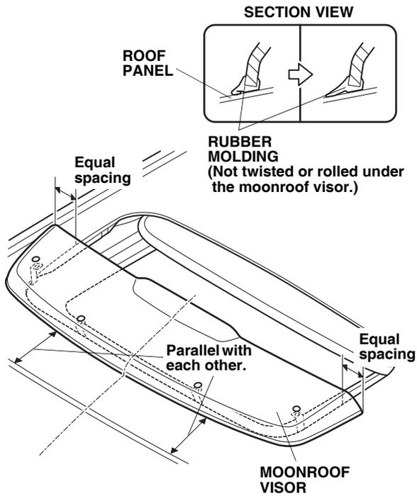
14. Tighten two screws and two nuts on the sides of the visor first, then tighten two screws and two nuts on the front. Tighten while applying pressure so that there is no gap between the roof panel and the brackets. Torque the screws to 2.0 N·m (1.5 lbf·ft).
