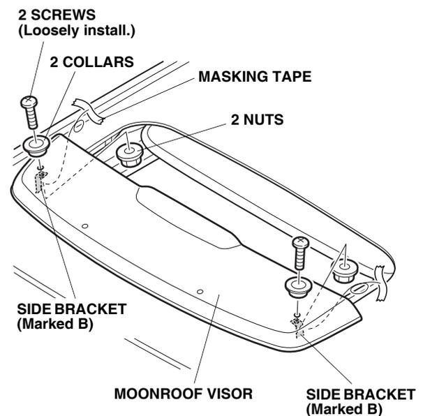
13. Position the moonroof visor with equal spacing on all sides. Check that the rubber molding is not twisted or rolled under the moonroof visor.
