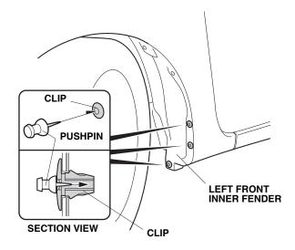
2. Using a pushpin, pierce the centers of three clips on the left front inner fender.
