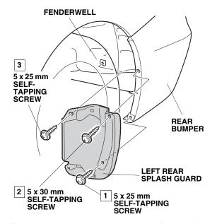
17. Repeat steps 12 through 16 to install the right rear splash guard on the right side of the vehicle.
