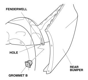
8. Reinstall the rear bumper onto the retaining tabs, and reinstall one self-tapping screw. Install one grommet A into the hole in the fenderwell.
