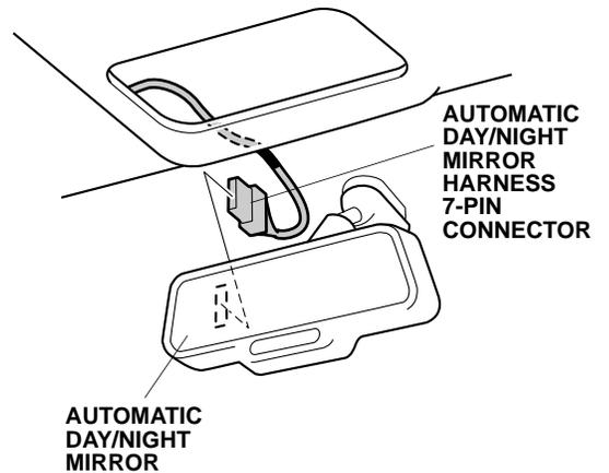
36. Align the green tape on the automatic day/night mirror harness at the headliner as shown. Route the automatic day/night mirror harness through the groove in the harness cover. Secure the harness cover to the mirror stay, and put the top of the harness cover behind the headliner.
