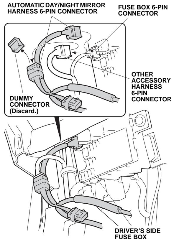
23. Plug the automatic day/night mirror harness 6-pin connector into the fuse box 6-pin connector.
