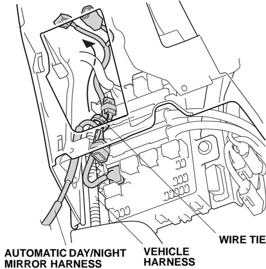
26. Secure the automatic day/night mirror harness to the vehicle harness with one wire tie.
