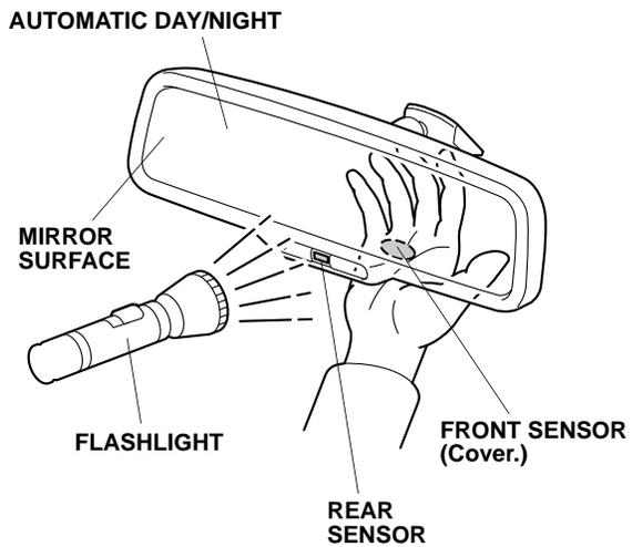
4. Make sure the parking brake is applied securely. Step on the brake pedal, and move the select lever to the "R" position. Repeat step 3, and make sure the mirror surface does not become dim.
