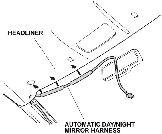
35. Plug the automatic day/night mirror harness 7-pin connector to the automatic day/night mirror.
