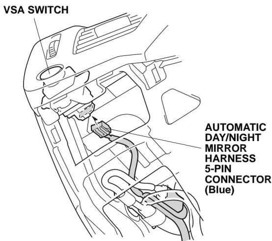
30. Using one wire tie, secure the automatic day/night mirror harness to the vehicle harness as shown.
