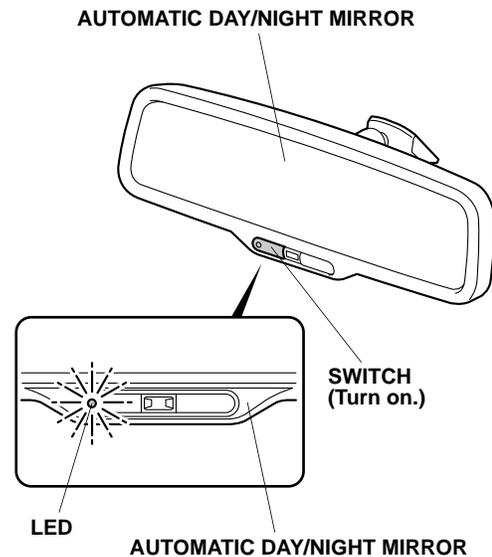
3. Cover the front sensor in the automatic day/night mirror with your hand, and use a flashlight on the rear sensor in the automatic day/night mirror. Make sure the mirror surface becomes dim.
