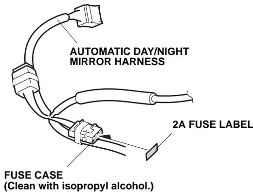
20. Attach the 2A fuse label to the fuse case on the automatic day/night mirror harness.
