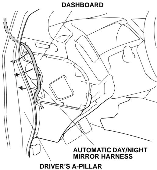
33. Align the green tape on the automatic day/night mirror harness with the vehicle clip, and secure the automatic day/night mirror harness to the vehicle harness with one wire tie.
