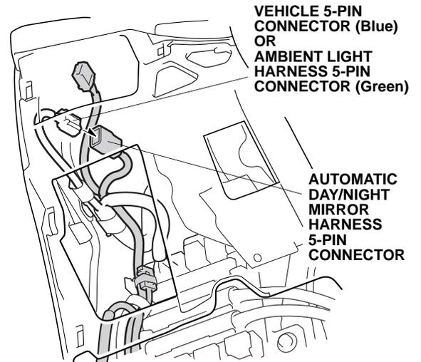
28. Unplug the vehicle 5-pin connector (blue) or, if equipped, the ambient light harness 5-pin connector (green) from the VSA switch, and plug it into the automatic day/night mirror harness 5-pin connector.
