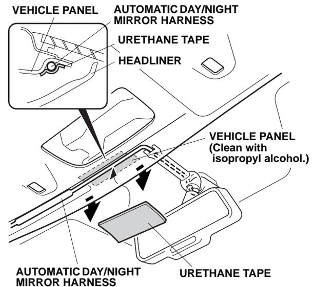
38. Secure the automatic day/night mirror harness to the vehicle panel with one urethane tape as shown. Be careful not to crease the headliner.
