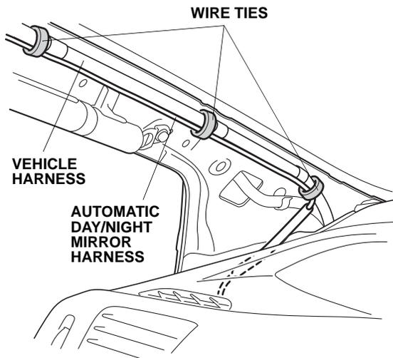
40. Non-Si models only: Plug the automatic day/night mirror harness 5-pin connector (blue) to the VSA switch.
