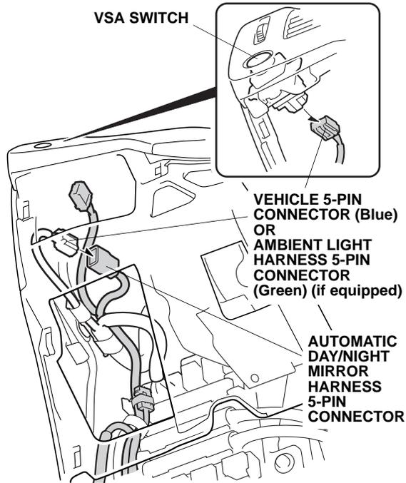
29. Plug the automatic day/night mirror harness 5-pin connector (blue) to the VSA switch.
