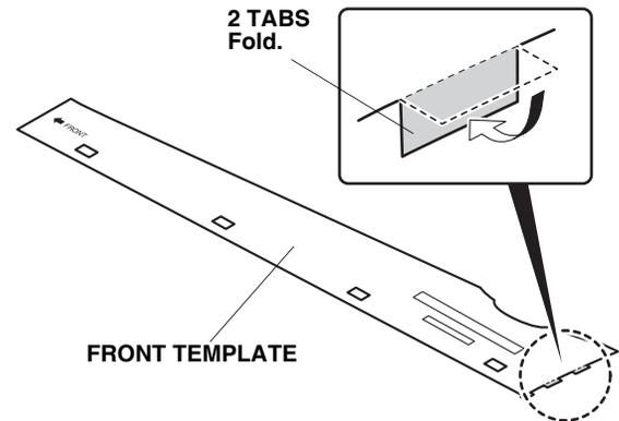
2. Insert the two tabs on the front template around the rear edge of the left front door.
