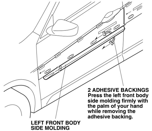
11. Using the rubber roller, apply firm pressure, especially at the ends, while rolling to set the adhesive.
