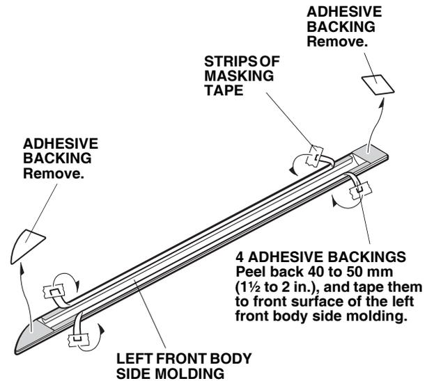
9. Align the edges of the left front body side molding with the edges of the front template, and install the left front body side molding on the left front door.
