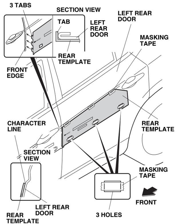
6. Align the rear template with the character line on the left rear door, and attach the rear template to the left rear door using strips of masking tape.
