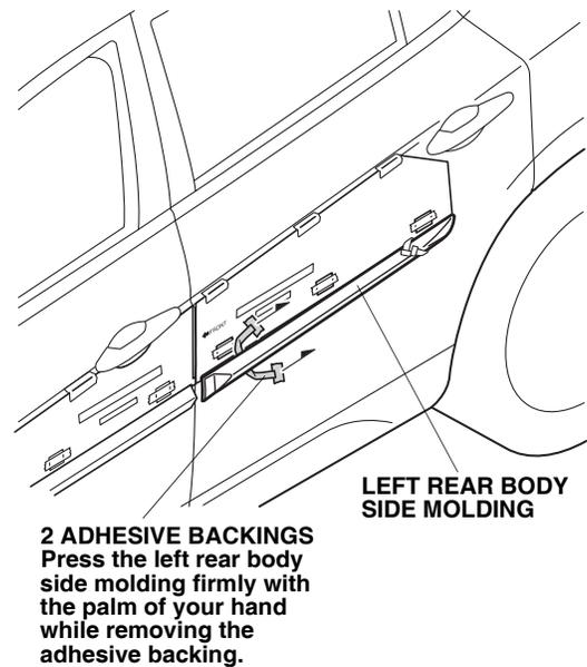
15. Using the rubber roller, apply firm pressure, especially at the ends, while rolling to set the adhesive.
