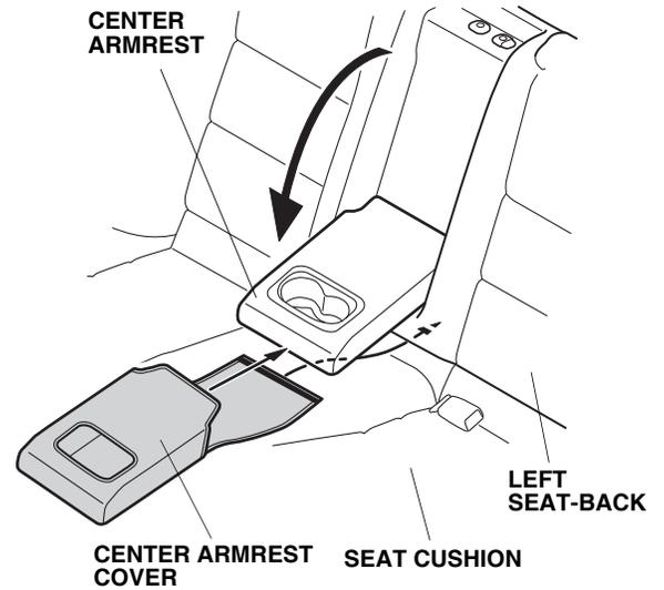
5. Fit the corners of the center armrest cover around the center armrest, and adjust the center armrest cover so it fits smoothly over the edges.
