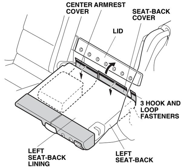
12. Repeat steps 7 thru 11 to install the seat-back cover on the right seat-back.
