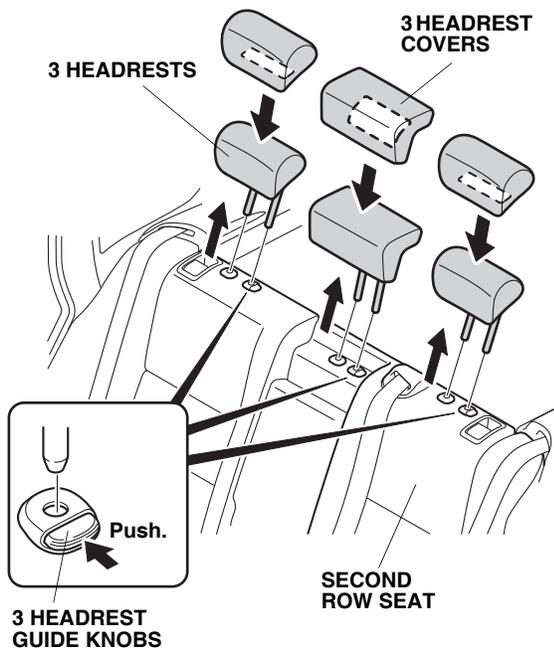
2. With the tag facing forward, fit the corners of the headrest cover around the headrest, and adjust the headrest cover so it fits smoothly over the edges.
