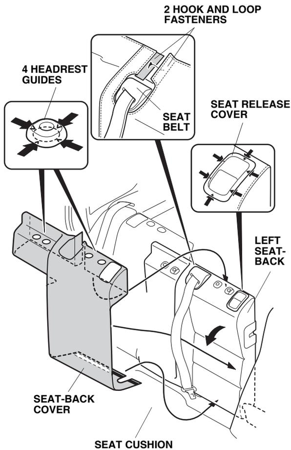
8. Route the seat-back cover under the seat belt, and secure the two hook and loop fasteners.
