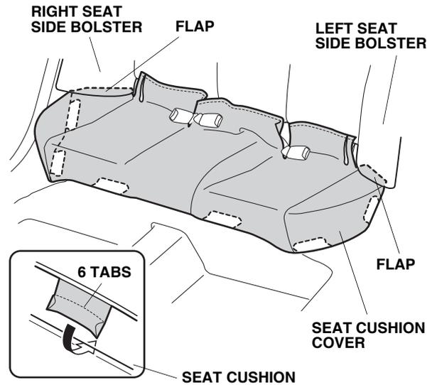
17. Fit the corners of the seat cushion cover around the seat cushion. Tuck the six tabs into the bottom of the seat cushion and tuck the two flaps between the seat cushion and each seat side bolster.
