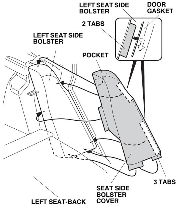
14. Slide the upper pocket over the top corner of the left seat side bolster. Starting from the top, slide the tabs downward, and insert the outer two tabs between the left seat side bolster and the door gasket. Install the remaining three tabs, and adjust the seat side bolster cover so it fits smoothly over the edges.
