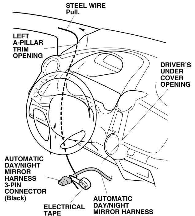
20. Use the steel wire to route the automatic day/night mirror harness up the left A-pillar trim opening. Remove the electrical tape and the steel wire from the automatic day/night mirror harness.
