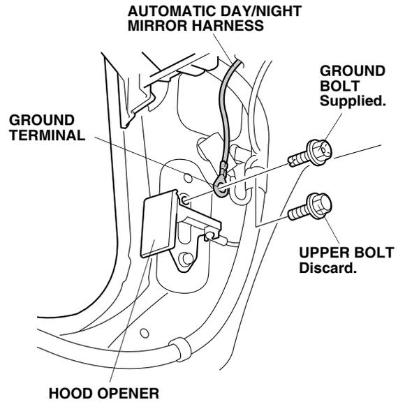
31. Secure the automatic day/night mirror harness to the vehicle harness with three wire ties.
