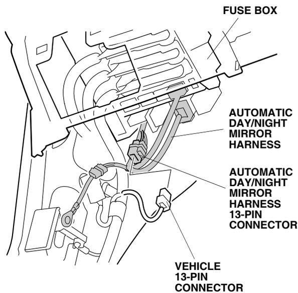
30. Remove and discard the upper bolt from the hood opener, and install the supplied ground bolt with the automatic day/night mirror harness ground terminal attached.
