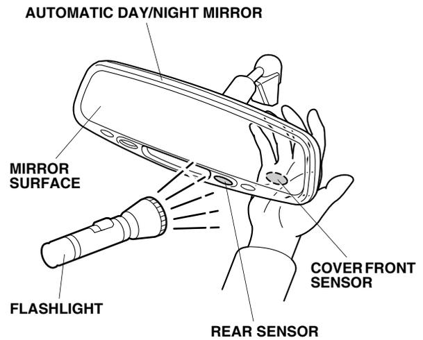
4. Step on the brake pedal, and move the shift lever to the "R" position. Repeat step 3, and make sure the mirror surface does not dim.
