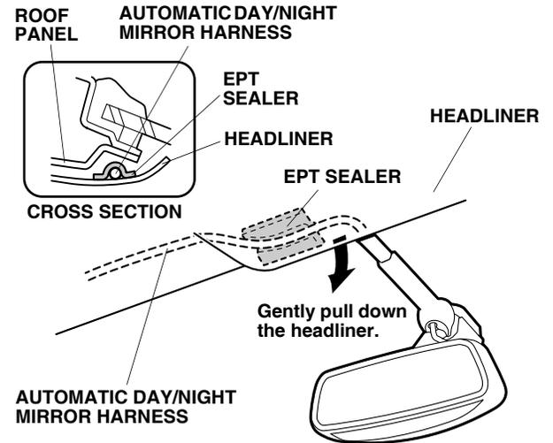
26. Route the automatic day/night mirror harness in front of the vehicle harness. Secure the mirror harness with four additional wire ties positioned as shown.
