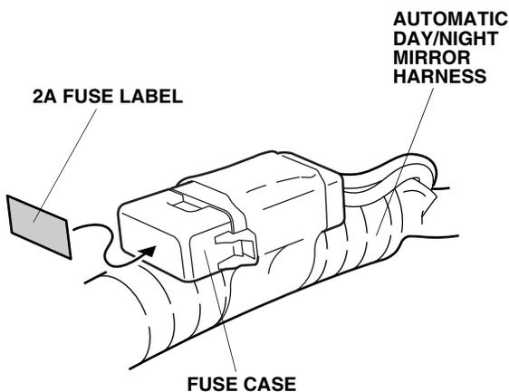
19. Use electrical tape to attach a piece of steel wire to the black connector on the automatic day/night mirror harness.
