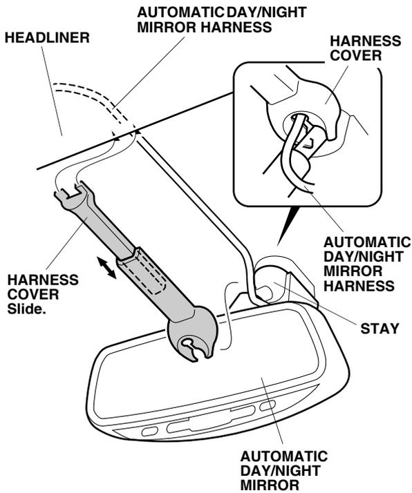
25. Secure the automatic day/night mirror harness to the headliner with one EPT sealer:
