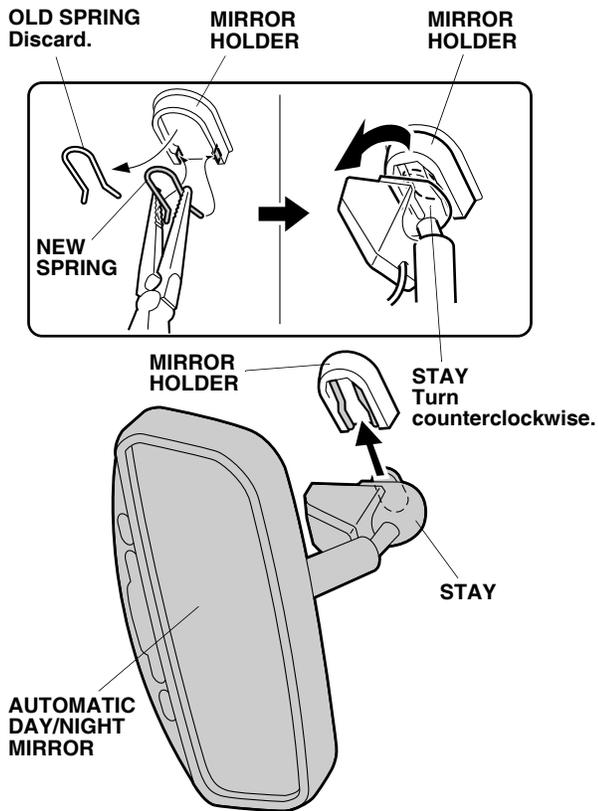
17. Slide the stay on the automatic day/night mirror into the mirror holder, and rotate the stay counterclockwise to secure the mirror.
