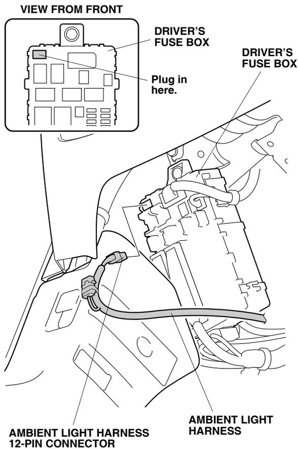
8. Secure the ambient light harness to the vehicle harness with one wire tie.
