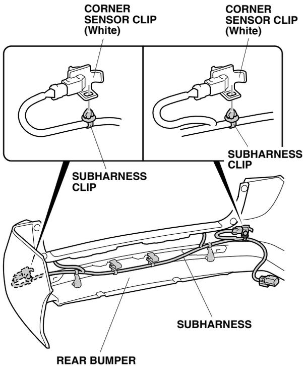
26. Secure two subharness clips to the two holes in the rear bumper as shown.
