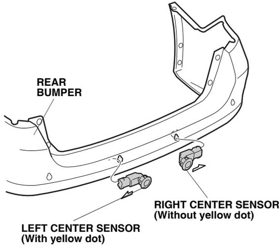
21. On the inside of the rear bumper, install the right center sensor clip (black) and left center sensor clip (white) to the right center sensor and left center sensor.
