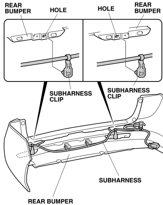
27. Secure two subharness clips to the two ribs on the rear bumper as shown.
