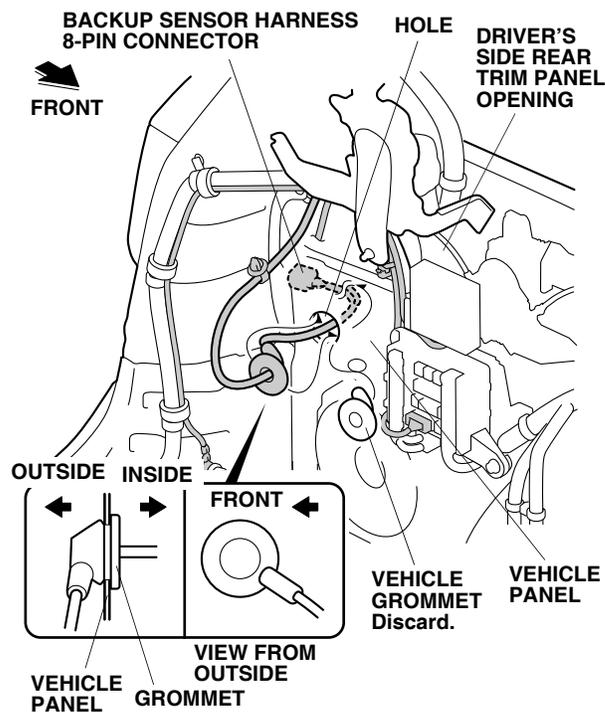
66. Route the backup sensor harness 8-pin connector through the hole, and seat the backup sensor harness grommet into the vehicle panel as shown. Do not pull on the backup sensor harness when installing the grommet.
