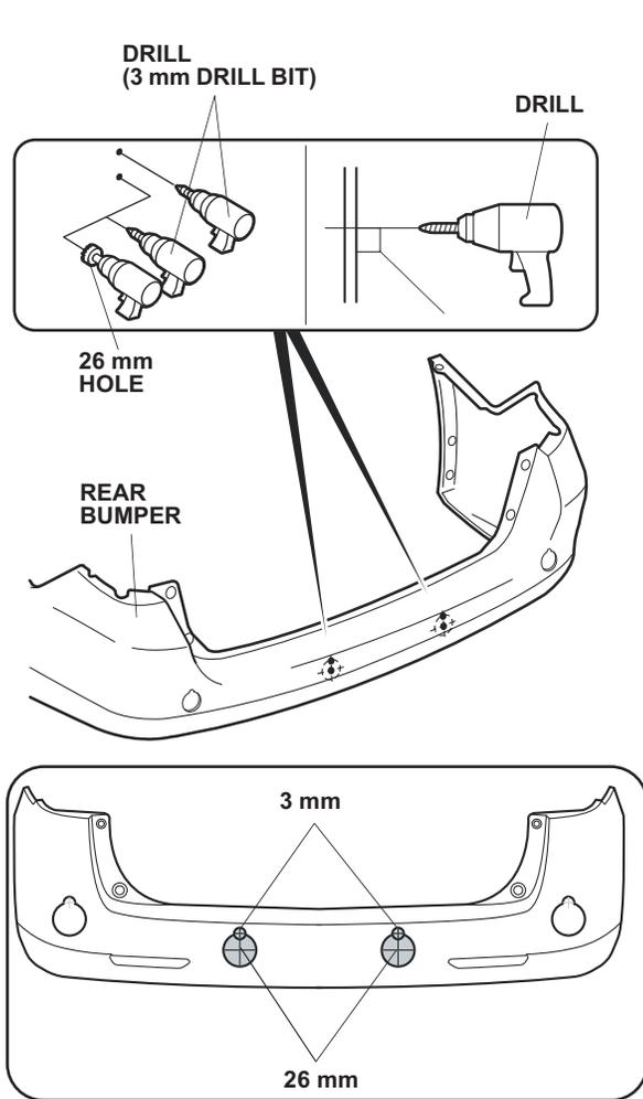
19. While wearing eye protection, drill the outer surface with a 3 mm drill bit at the four pierced marks in the corners of the rear bumper. Enlarge the two lower holes with a 24 mm hole saw. Remove any burrs.
