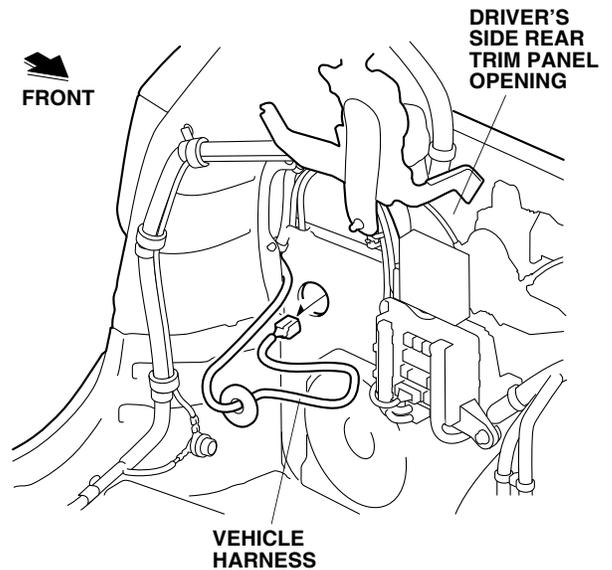
59. Route the backup sensor harness 8-pin connector through the hole, and seat the backup sensor harness grommet into the vehicle panel as shown. Do not pull on the backup sensor harness when installing the grommet.
