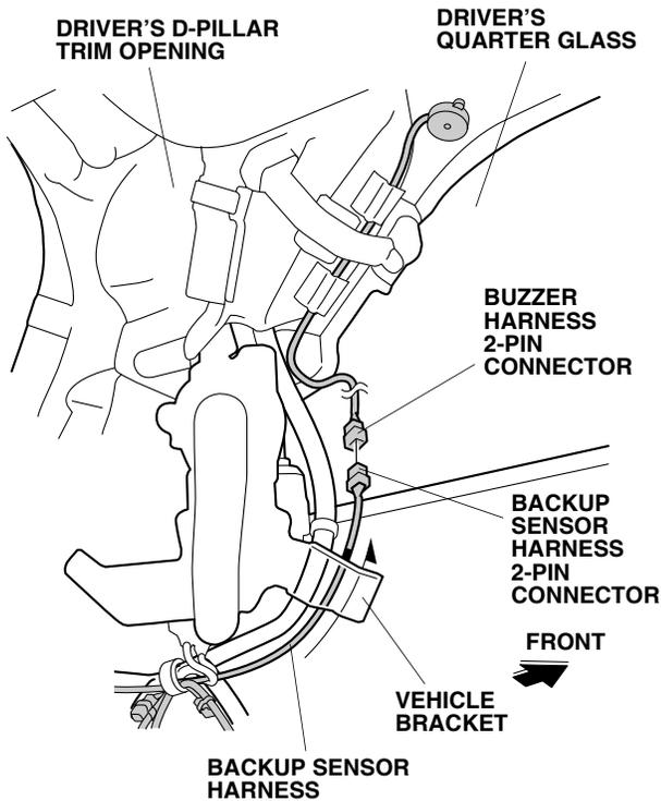
43. Plug the backup sensor harness 2-pin connector into the buzzer harness 2-pin connector.
