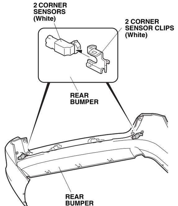
24. Plug the four backup sensor subharness 2-pin connectors into the right center sensor, left center sensor, and two corner sensors.
