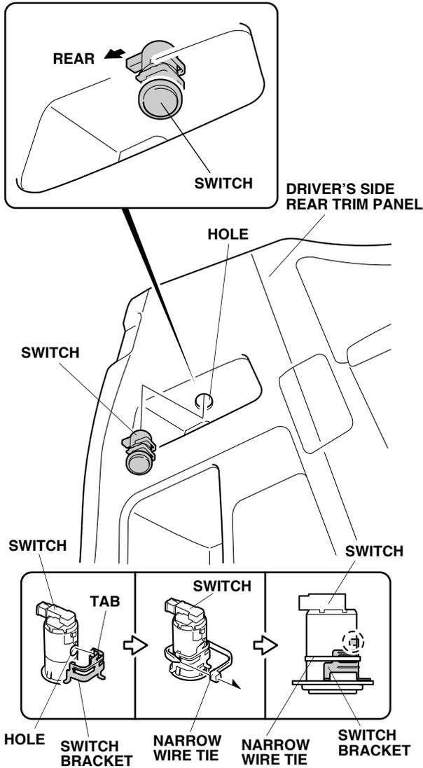
31. Align the tab on the switch bracket to the hole on the switch and secure the switch bracket to the switch with one narrow wire tie.
