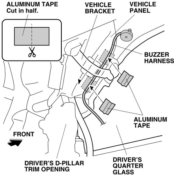
35. Using isopropyl alcohol on a shop towel, thoroughly clean the areas where the aluminum tapes will attach.
