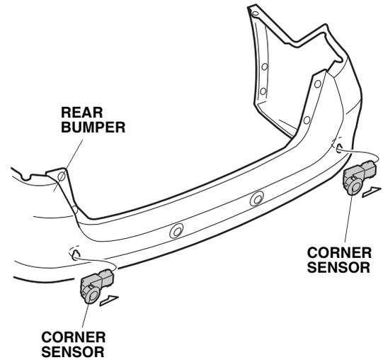
23. On the inside of the rear bumper, install the two corner sensor clips (white) to the two corner sensors.
