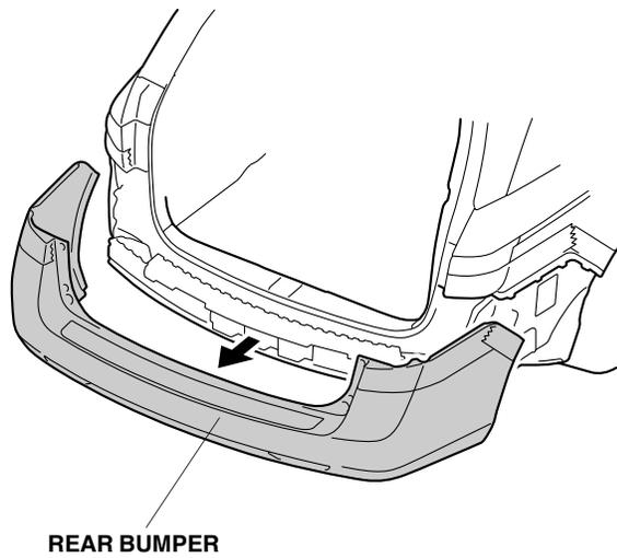
17. On the inside of the rear bumper, locate and pierce the eight scribe marks using a pushpin. Make sure to pierce the scribe marks perpendicularly to the rear bumper.
