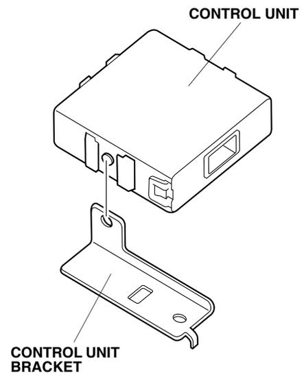
53. Align the control unit bracket to the holes in the vehicle bracket, and secure it to the vehicle bracket with one flange bolt.
