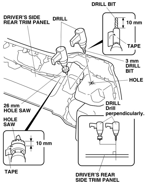
30. Install the switch into the driver's side rear trim panel.
