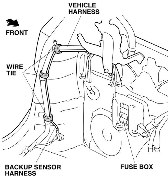
42. Route the backup sensor harness 2-pin connector along the vehicle harness.
