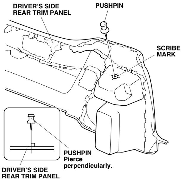
29. While wearing eye protection, drill a 26 mm hole through the pierced mark. Make sure to drill perpendicularly to the driver's side rear trim panel. Be careful not to damage the driver's side rear trim.
