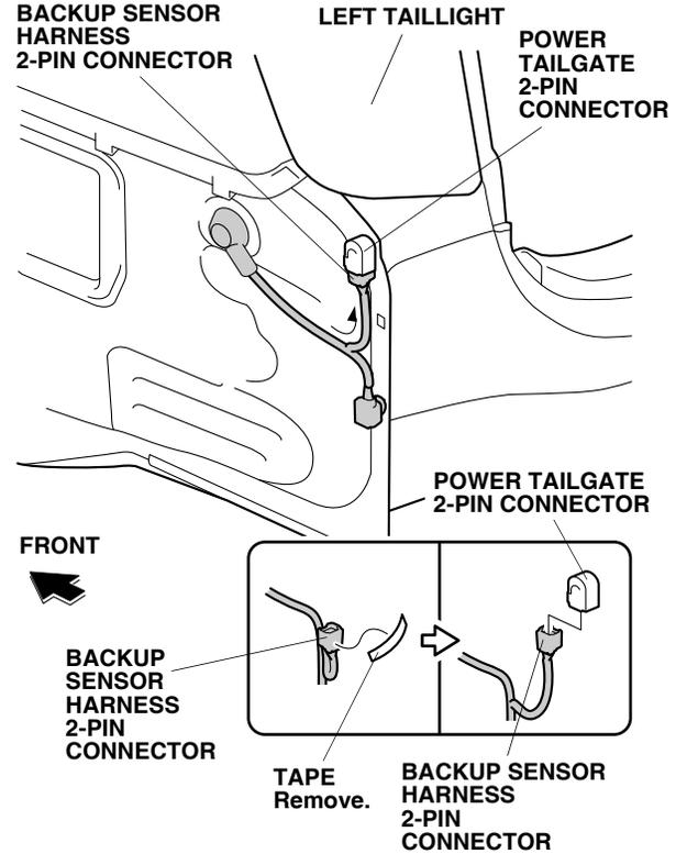
62. Route the vehicle 2-pin connector as shown, and plug it to the backup sensor harness 2-pin connector.
