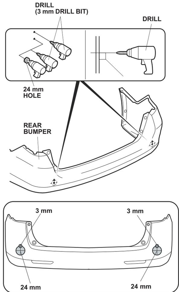
20. From the outside of the rear bumper, insert the right center sensor (**without** yellow dot) and left center sensor (**with** yellow dot) into the 26 mm holes that you drilled. Make sure the detent on each sensor points upward and locks into the 3 mm hole that you drilled, and that the connector faces outward.
