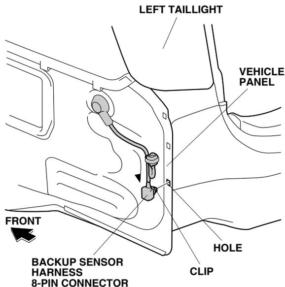
68. Secure the clip on the backup sensor harness to the hole in the vehicle panel as shown.
