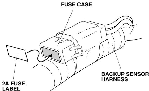
38. Secure the backup sensor harness to the vehicle harness with one wire tie as shown.
