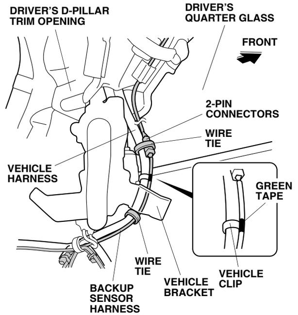
45. Secure the backup sensor harness to the vehicle harness with one wire tie.
