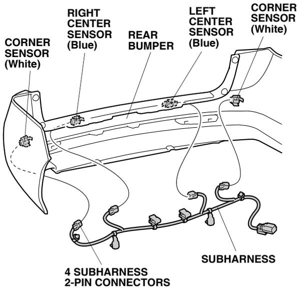
25. Secure two subharness clips to the two corner sensor clips (white) as shown.
