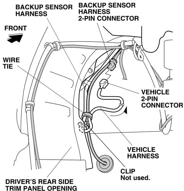
63. Secure the vehicle harness and backup sensor harness to the vehicle harness with one wire tie as shown.
