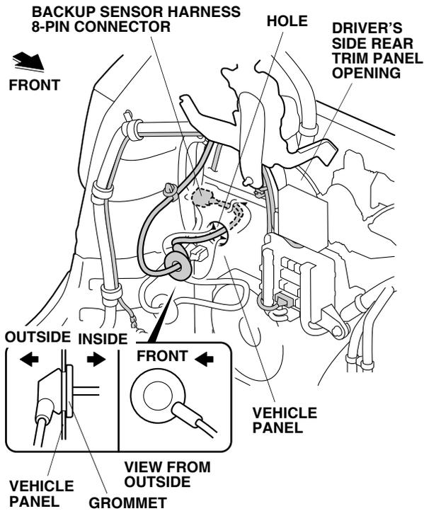
60. Route the backup sensor harness 8-pin connector down, and secure the clip on the 8-pin connector into the hole in the vehicle panel.
