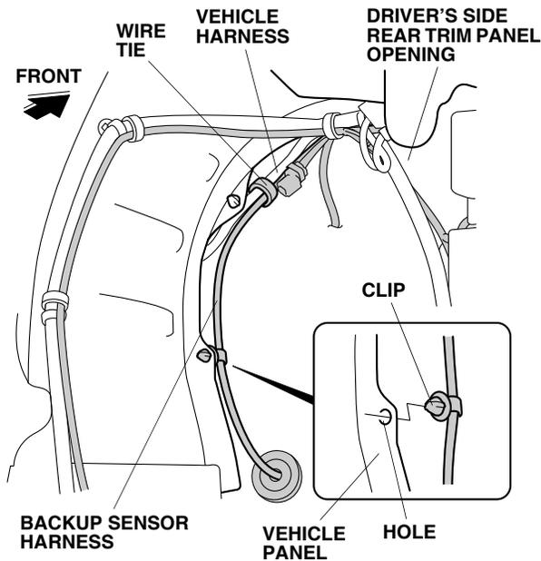
69. Secure the backup sensor harness to the vehicle harness with one wire tie.
