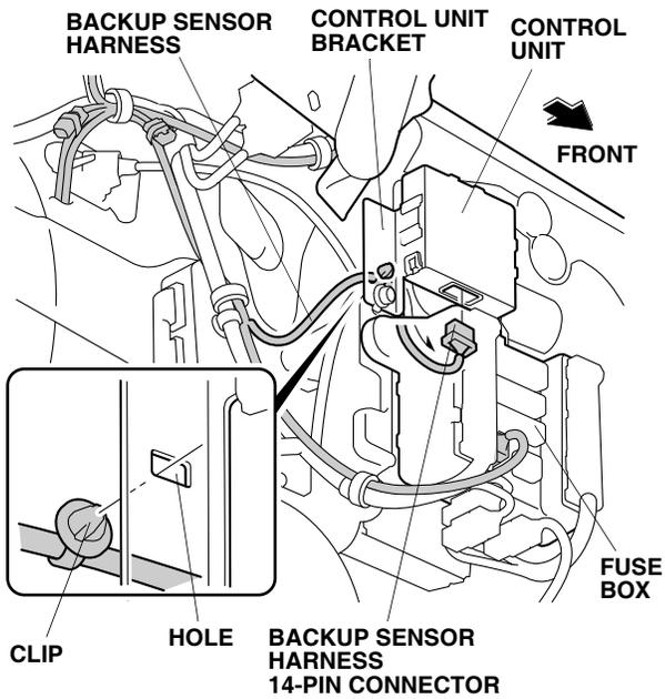
55. Secure the clip on the backup sensor harness to the hole in the control unit bracket as shown.
