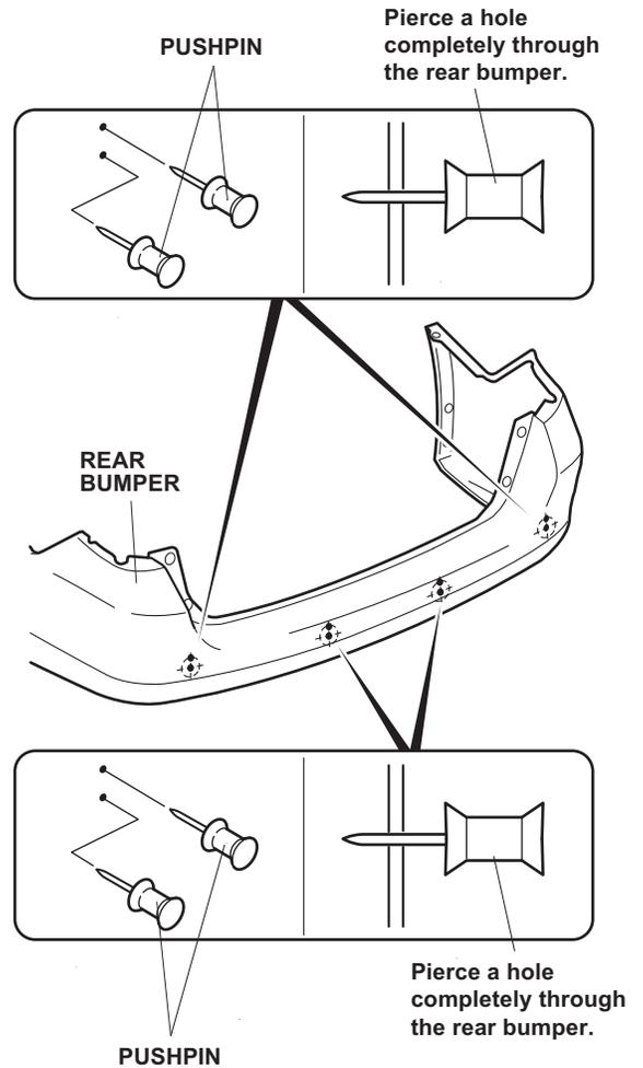
18. While wearing eye protection, drill the outer surface with a 3 mm drill bit at the four pierced marks in the center section of the rear bumper. Enlarge the two lower holes with a 26 mm hole saw. Remove any burrs.
