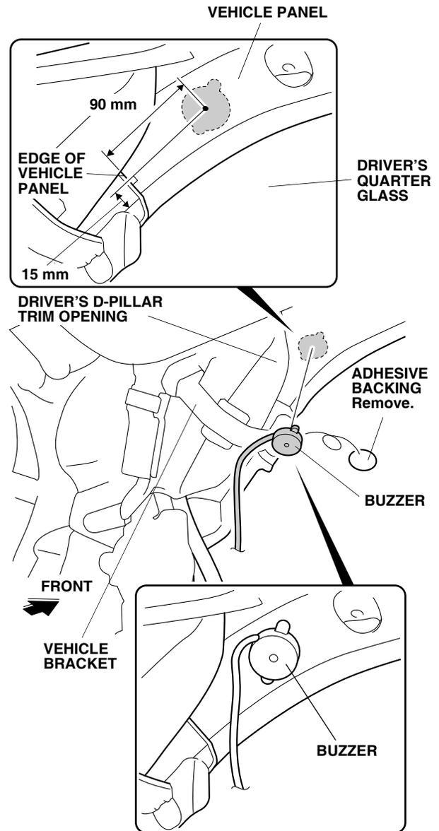
33. Remove the adhesive backing from the buzzer and attach it to the vehicle panel in the location shown.
