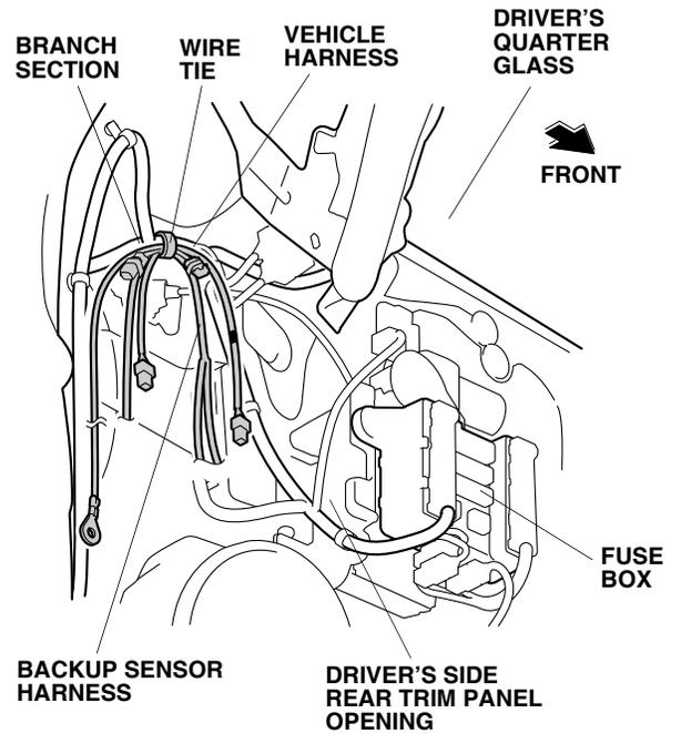
39. Route the backup sensor harness ground terminal along the vehicle harness.
