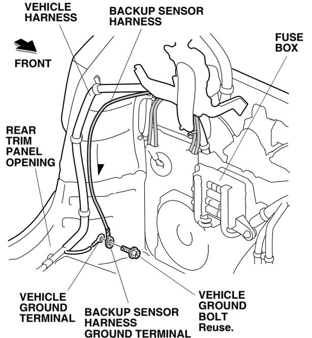
40. Remove the vehicle ground bolt. Secure the backup sensor harness ground terminal to the vehicle ground terminal with the vehicle ground bolt you just removed.
