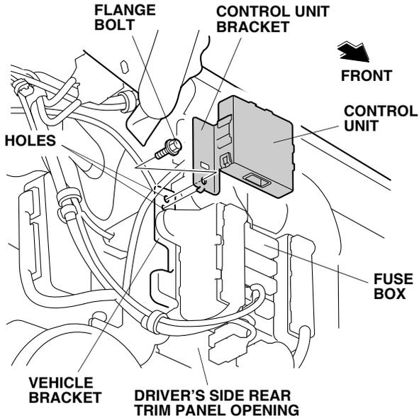
54. Route the backup sensor harness 14-pin connector, and plug it to the control unit.
