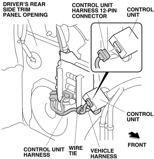
25. Secure the control unit harness to the vehicle harness with one wire tie.
