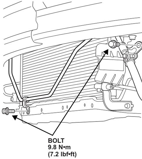
57. Detach the clips, then remove the left air guide.
