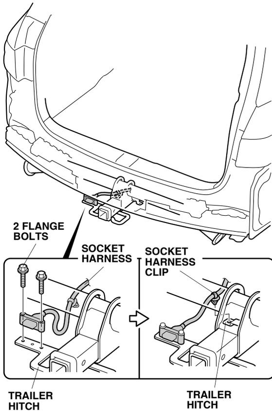
43. Secure the socket harness to the trailer hitch with the socket harness clip.
