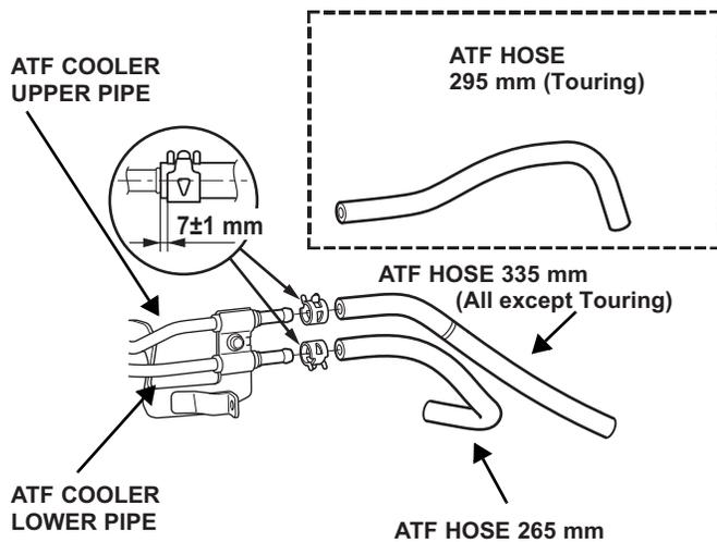
61. Route the hoses installed on the ATF cooler through the hole cut in the left air guide, and fit the ATF cooler into place on the bulkhead. Install the three washer-bolts from the kit through the ATF cooler into the threaded holes in the front bulkhead. Tighten the bolts securely.
