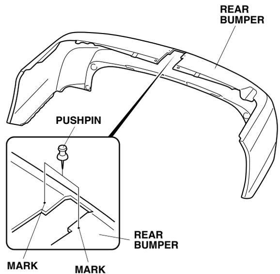
39. While wearing eye protection, drill the rear bumper. First drill with a 3 mm drill bit, and finish with a 10 mm drill bit. Remove any burrs.
