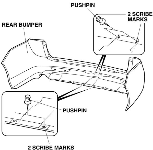
32. While wearing eye protection, drill the front two pierced marks in the rear bumper. First drill with a 3 mm drill bit, and finish with a 10 mm drill bit. Remove any burrs.
