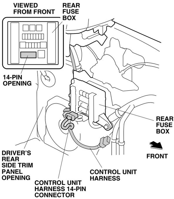
21. Install the control unit onto the control unit bracket.
