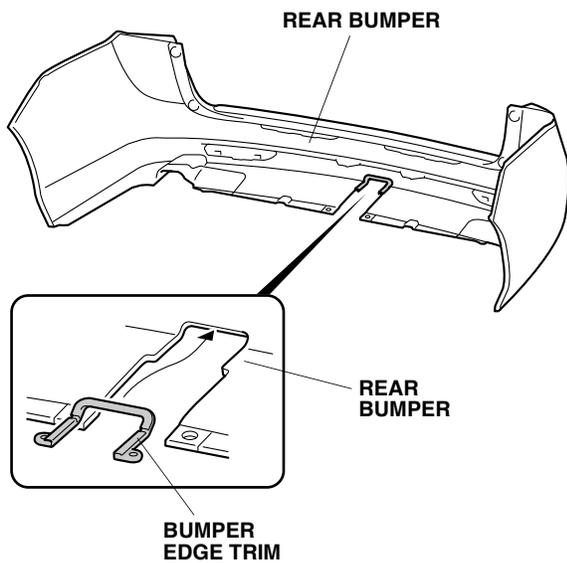
36. Using a felt-tip pen, mark the centers of the bumper edge trim holes.
