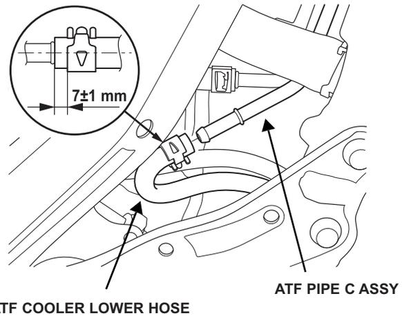
64. *All except Touring:* Attach the hose spacer between the two hoses at the white paint on the ATF hose.
