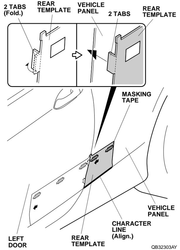
4. Insert the folded tabs of the rear template into the opening between the left door and the vehicle panel. Align the template with the character line, and tape the template to the vehicle panel with strips of masking tape.
