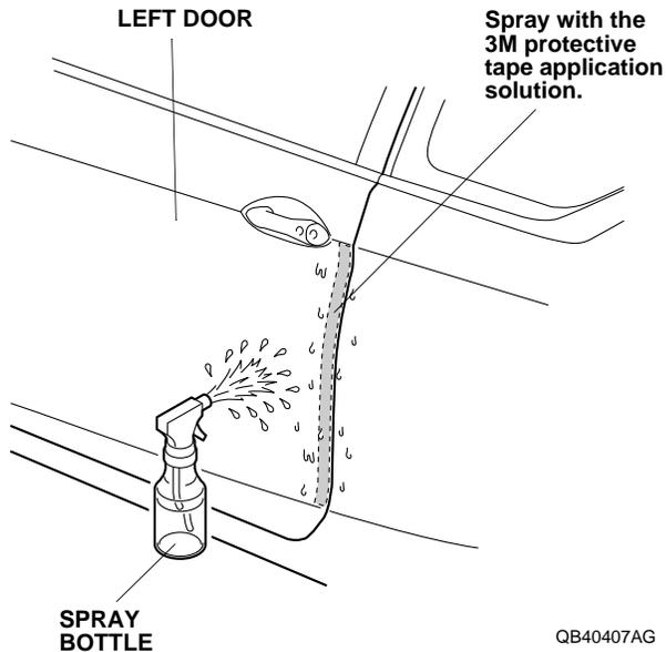
4. Open the left door. Peel back about 50 mm (2.0 in.) of adhesive backing from the left door edge film. Align the V-notch on the left door edge film 45 mm (1.8 in.) below the character line.
