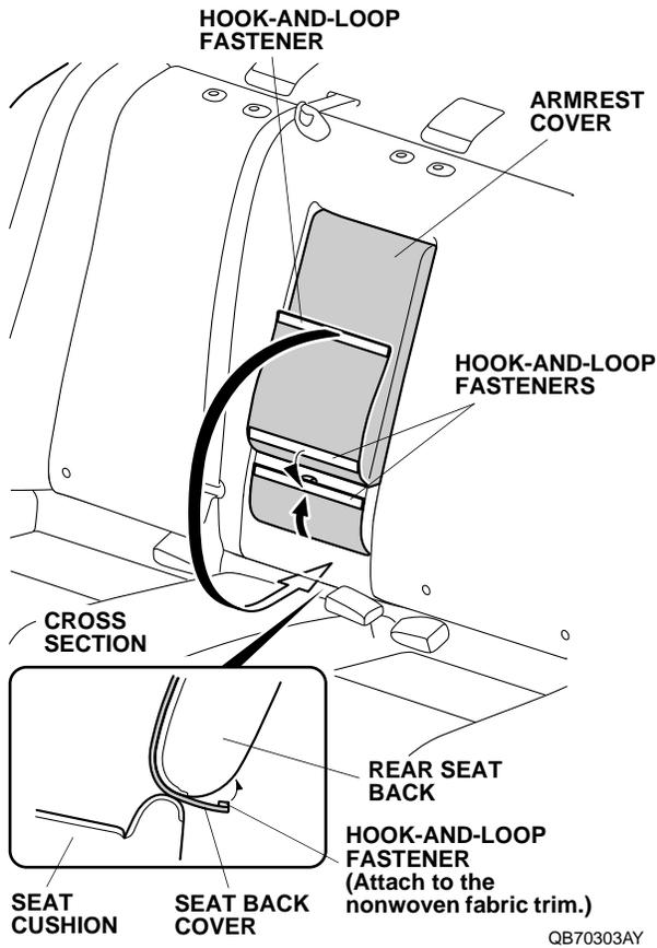
15. Insert the armrest cover between the rear seat back and the rear seat cushion, secure the hook-and-loop fastener to the rear seat back.
