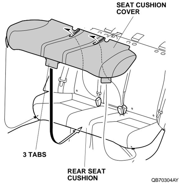
17. Insert the seat cushion cover between the rear seat back and the rear seat cushion, and secure the three hook-and-loop fasteners to the rear seat cushion.
