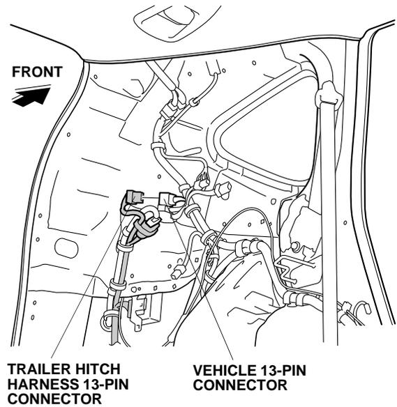
46. Plug the backup sensor harness 13-pin connector into the vehicle 13-pin connector.
