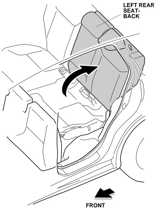
5. Remove the left rear door sill trim (three clips, five retaining tabs, and one hook).
