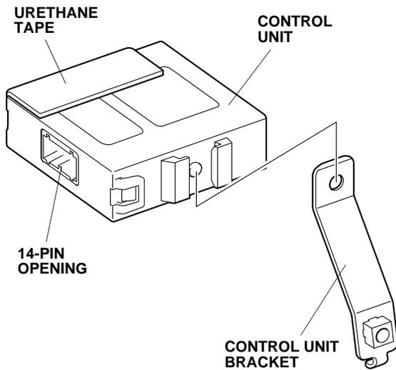
35. Using isopropyl alcohol on a shop towel, thoroughly clean the control unit where the urethane tape will attach. Attach the remaining half of urethane tape (cut in step 33) to the control unit in the area shown.
