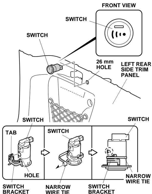
60. Align the tab on the switch bracket with the hole in the switch, and secure the switch bracket to the switch with one narrow wire tie. Firmly press the switch bracket against the left rear side trim panel, and make sure there is no clearance between the switch and the left rear side trim panel.
