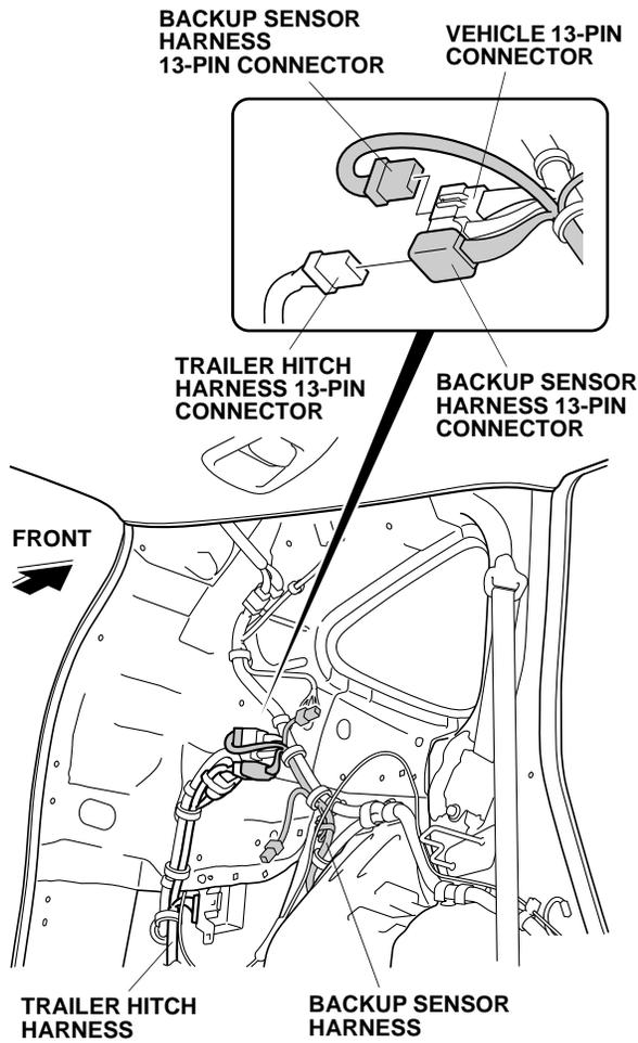
47. Plug the trailer hitch harness 13-pin connector into the backup sensor harness 13-pin connector. Go to step 50.
