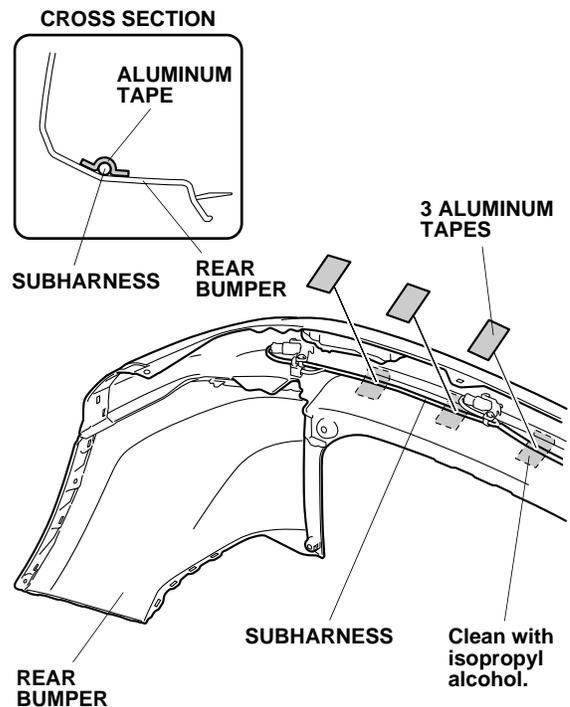
78. Secure the subharness to the rear bumper with three aluminum tapes in the areas shown.
