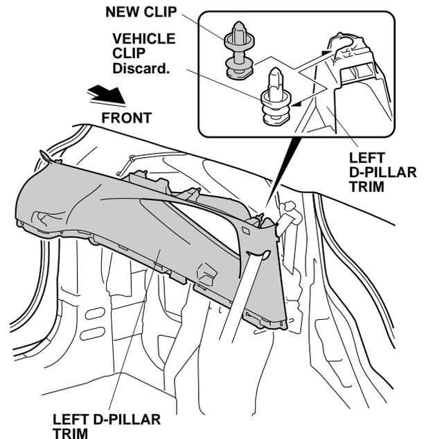
62. Check the overlap between the headliner and the D-pillar trim. If necessary, adjust the overlap as shown in the service manual.
