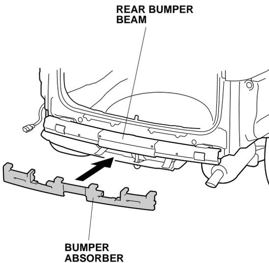
81. With the help of an assistant, bring the rear bumper to the vehicle, and plug the backup sensor harness 8-pin connector into the subharness 8-pin connector. Reinstall the rear bumper.
