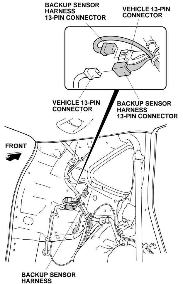
49. Plug the vehicle 13-pin connector into the backup sensor harness 13-pin connector.
