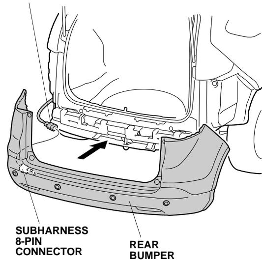
82. Check that all wire harnesses are routed properly and that all connectors are plugged in.
