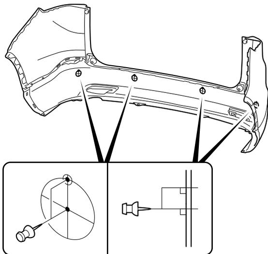
66. While wearing eye protection, drill the eight pierced marks with a 3 mm drill bit. Work from the painted side of the rear bumper. Drill perpendicular to the rear bumper.
