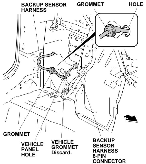
30. Route the backup sensor harness 8-pin connector through the hole, and set the backup sensor harness grommet into the vehicle panel hole. Do not pull on the backup sensor harness.
