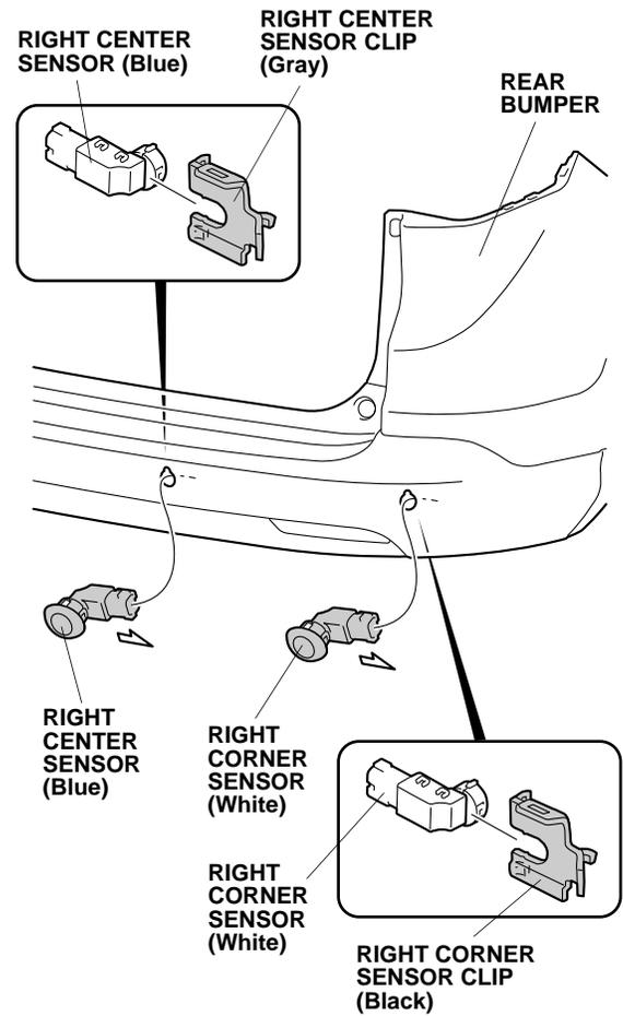
72. Secure the right corner sensor (white) and the right center sensor (blue) with the right corner sensor clip (black) and the right center sensor clip (gray) as shown.
