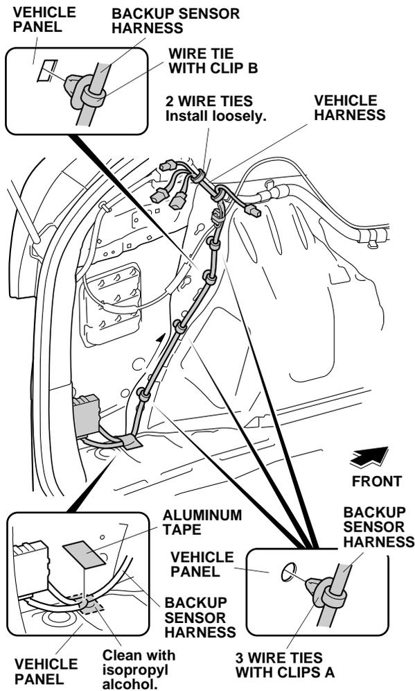
41. Route the backup sensor harness along the vehicle harness. Secure it to the vehicle panel and vehicle harness with three wire ties with clips A, one wire tie with clip B, and two loosely-installed wire ties.
