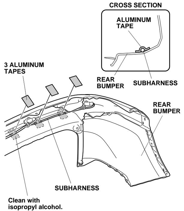
76. Secure the subharness to the rear bumper with three aluminum tapes at the areas shown.
