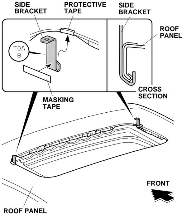
11. Place one front bracket into position over the protective tape, and align the lower edge with the indentation on the roof panel. Tape the bracket in position with a piece of masking tape. Repeat the same procedure to install the other front bracket on the moonroof opening.
