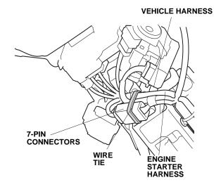
76. Route the engine starter harness across the steering column area as shown.
