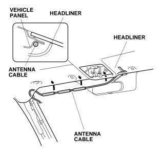
34. Using isopropyl alcohol on a shop towel, thoroughly clean the vehicle panel, where the urethane tapes will attach.
