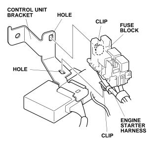
91. Remove the vehicle flange nut that secures the vehicle bracket.
