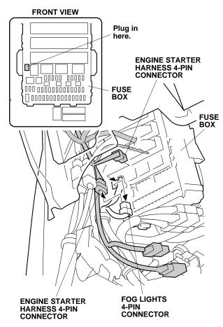
55. Plug the remaining engine starter harness 4-pin connector into the fuse box.
