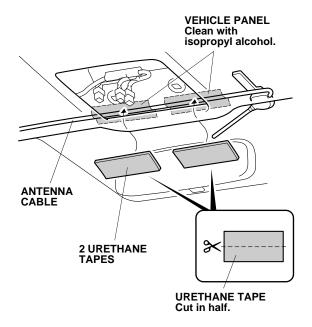
35. Using scissors, cut one urethane tape in half. Secure the antenna cable to the vehicle panel with two cut pieces of urethane tape. Be careful not to crease the headliner.
