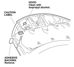
99. Remove the adhesive backing from the caution label, and attach the caution label to the hood in the area shown.
