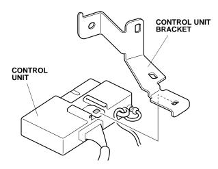
90. Secure the clip from the engine starter harness fuse block, and the clip from the engine starter harness into the holes in the control unit bracket.
