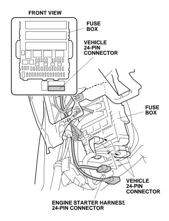
66. Slide the clip from the engine starter harness 24-pin connector onto the bottom of the fuse box, then plug the remaining vehicle 24-pin connector into the engine starter harness 24-pin connector.
