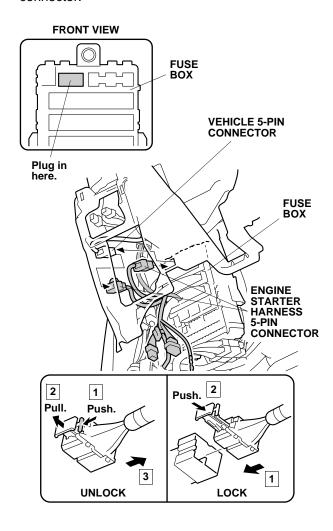
50. Plug the remaining engine starter harness 5-pin connector into the fuse box.
