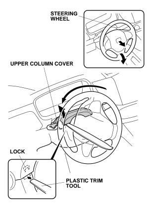
19. Using a plastic trim tool, release the lock as shown.
