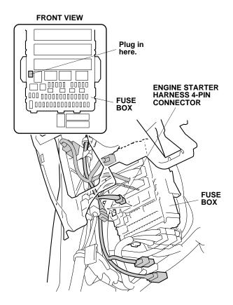
54. Unplug the fog light 4-pin connector from the fuse box, and plug it into the engine starter harness 4-pin connector.
