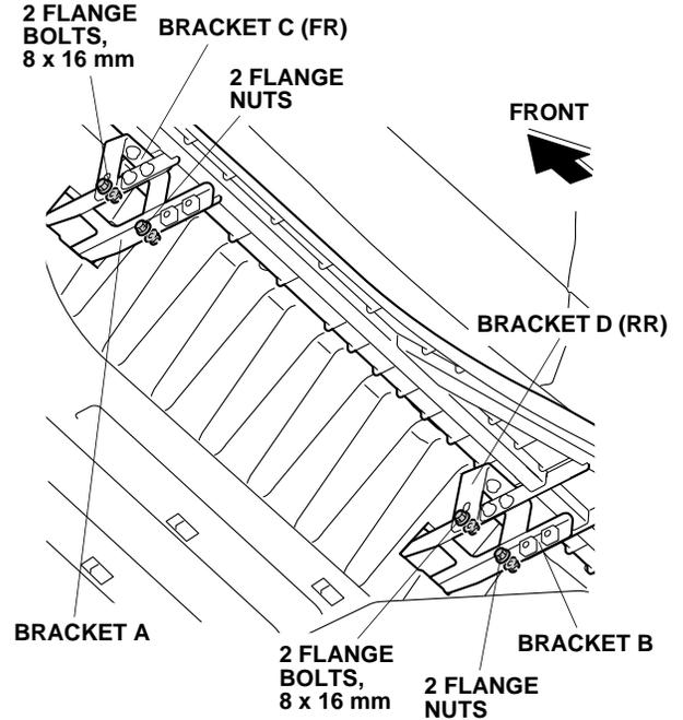
27. Torque the eight 8 x 16 mm flange bolts loosely installed in step 23 to 22 N·m (6 lbf·ft).
