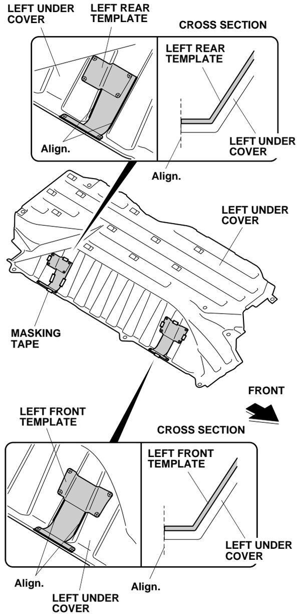
5. Using a pushpin, pierce the six marks on each template.
