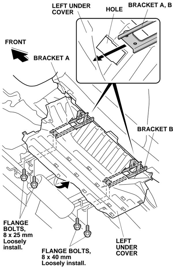
21. With the help of an assistant, bring the left under cover close to the vehicle and loosely install bracket A and bracket B to the vehicle panel using two 8 x 25 mm flange bolts and two 8 x 40 mm flange bolts.
