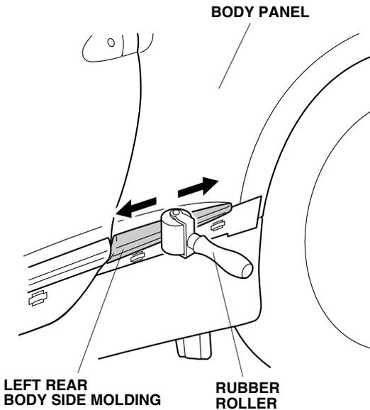
16. Turn the template over, and repeat steps 1 through 15 to install the body side moldings on the right side of the vehicle.
