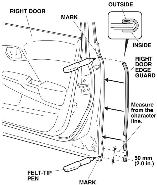
2. Using a felt-tip pen, mark the sealant at the top and bottom ending point of right door edge guard.
