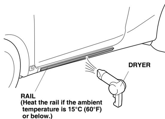
25. Using the palm of your hand, firmly press the rail against the vehicle panel.
