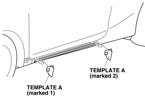
24. If the ambient air temperature is 15°C (60°F) or below, use a dryer to heat the surface of the rail to 15 - 40°C (60 - 104°F). The rail may not properly adhere to the vehicle otherwise.
