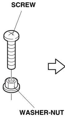
40. Using a Phillips screwdriver, securely tighten the screw into the clamp. Finger-tighten the washer-nut against the clamp. While holding the screw, tighten the washer-nut 90° clockwise with a 10 mm open end wrench.
