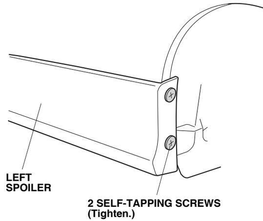
44. Tighten the bracket screw.
