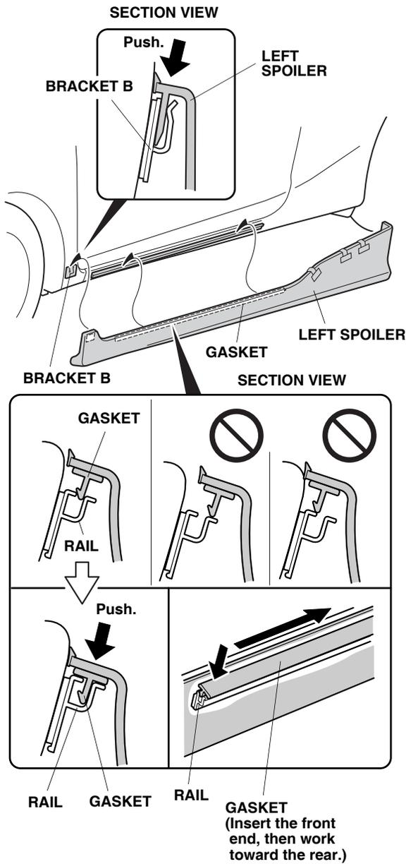
30. Lightly tap the left spoiler to make sure that there is no gap between the left spoiler and the left rear fenderwell.
