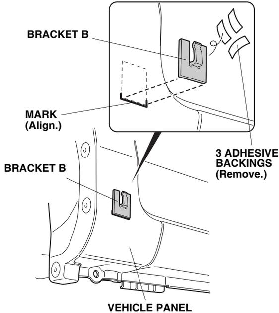
14. Align bracket B with the mark made in step 11, and attach it to the vehicle panel. Press firmly on bracket B firmly.
