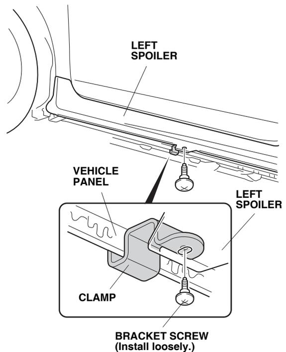
39. Assemble one screw and one washer-nut.
