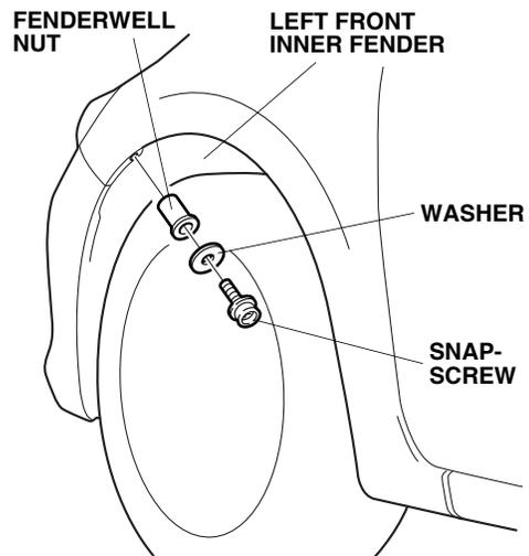
5. Place a washer onto the snap-screw and install one snap-screw into the fenderwell nut. Securely tighten the snap-screw.
