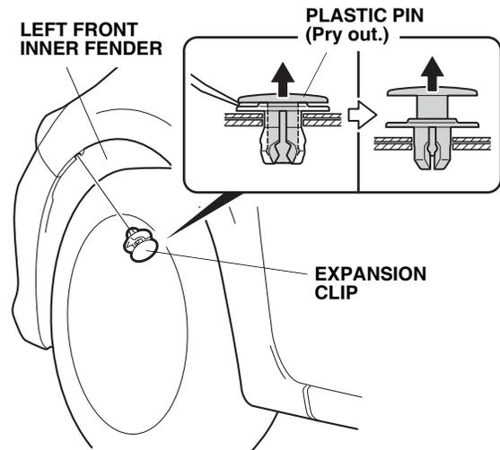
3. Pry out the plastic pin of clip, and remove the expansion clip that fastens the left front inner fender. Retain the clip. Clean the area around the hole.
