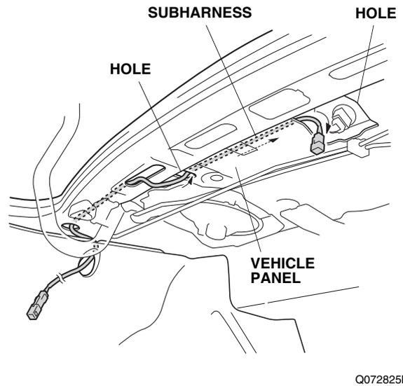
33. Unplug the vehicle 2-pin connector from the high-mount brake light connector.
