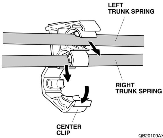
24. Put on heavy gloves to protect your hands. With an assistant holding the trunk lid open, remove both trunk springs with the trunk spring tool. Pull the trunk spring tool slowly and carefully toward you. First remove the right trunk spring, then remove the left trunk spring.
