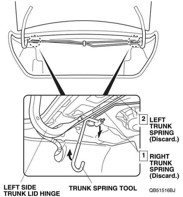
25. Install the new left and right trunk springs in the reverse order of removal:
