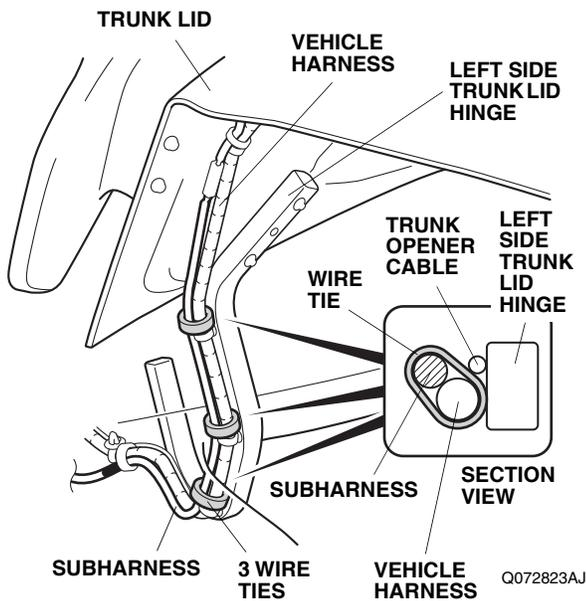
39. Check that all wire harnesses are routed properly and all connectors are plugged in.
