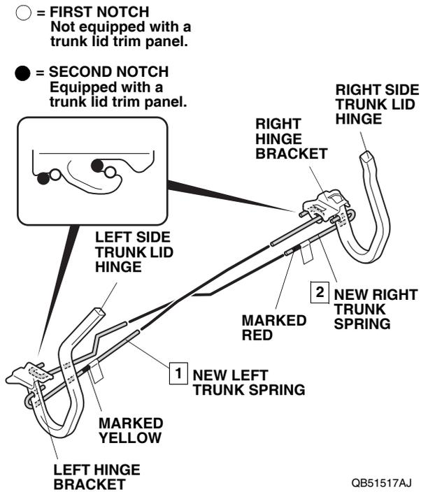
26. Reinstall the center clip to the trunk springs.
