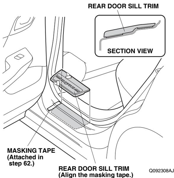
66. Attach the rear door sill trim to the vehicle panel by removing two adhesive backings and pressing on the trim firmly with your hands.
