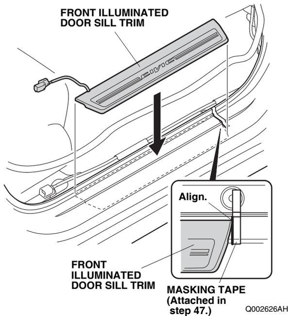
49. Route the front illuminated door sill trim harness over the vehicle panel of the door opening seal.
