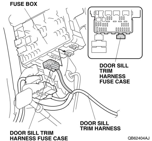
16. Secure the door sill trim harness to the vehicle harness with one wire tie.
