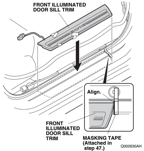
56. Attach the front illuminated door sill trim to the vehicle panel by removing three adhesive backings in the order shown and pressing on the trim firmly with your hands.
