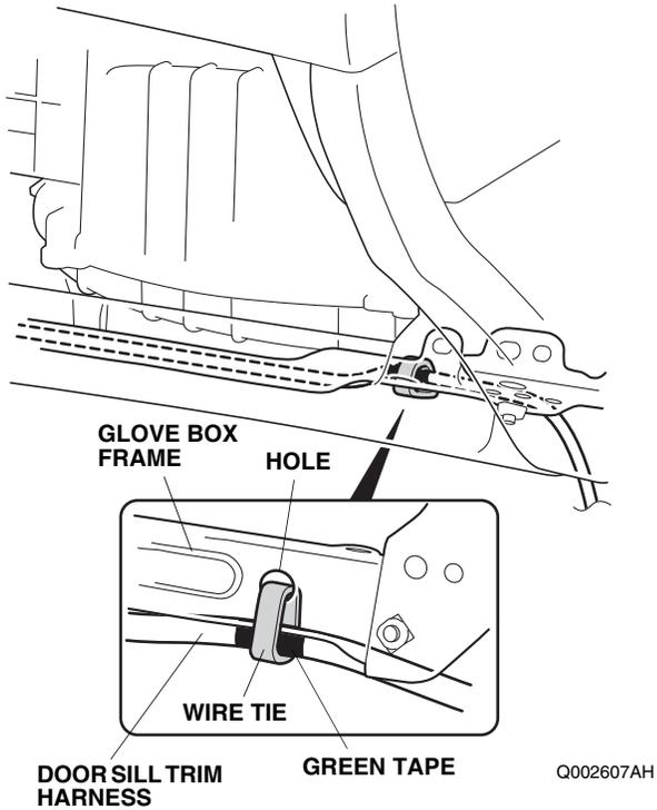
25. Secure the door sill trim harness to the glove box frame with one wire tie.
