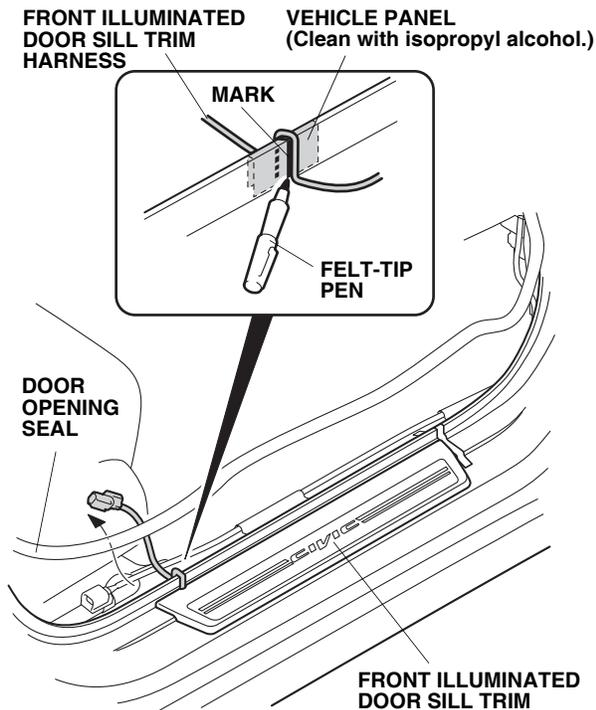
50. Using isopropyl alcohol on a shop towel, clean the vehicle panel around the harness, then use a felt-tip pen to mark the vehicle panel at the harness.
