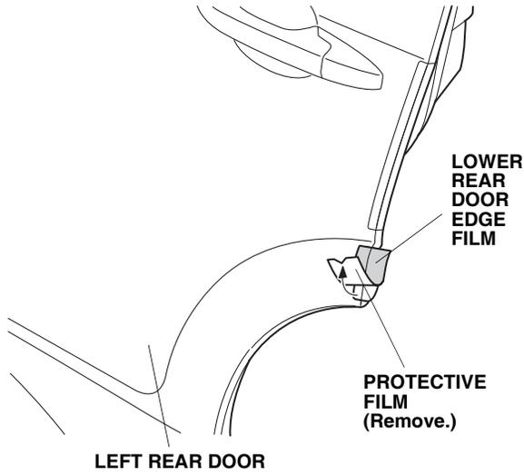
23. Starting from the middle of the lower door edge film and working outward, fold the door film around the edge using your fingers. Move your fingers in one direction. Attach the film over the seam sealant. Do not trim or damage the seam sealant.
