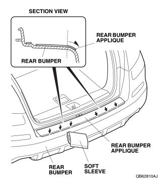
15. Using a shop towel, wipe away the excess 3M protective tape application solution. Allow the rear bumper applique to dry thoroughly.
