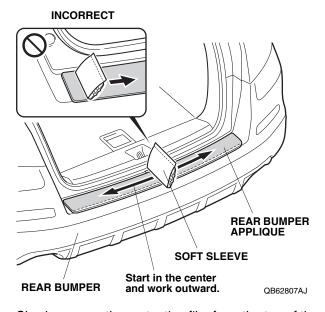
12. Slowly remove the protective film from the top of the rear bumper applique. Remove the protective film by pulling it slowly and horizontally; do not pull it vertically.
