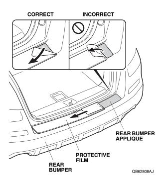
13. Repeat step 10 for the center of the lower section of the rear bumper applique.
