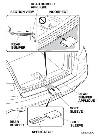
10. Starting from the center and working outward, use the soft sleeve to smooth out the center of the upper section on the rear bumper applique.
