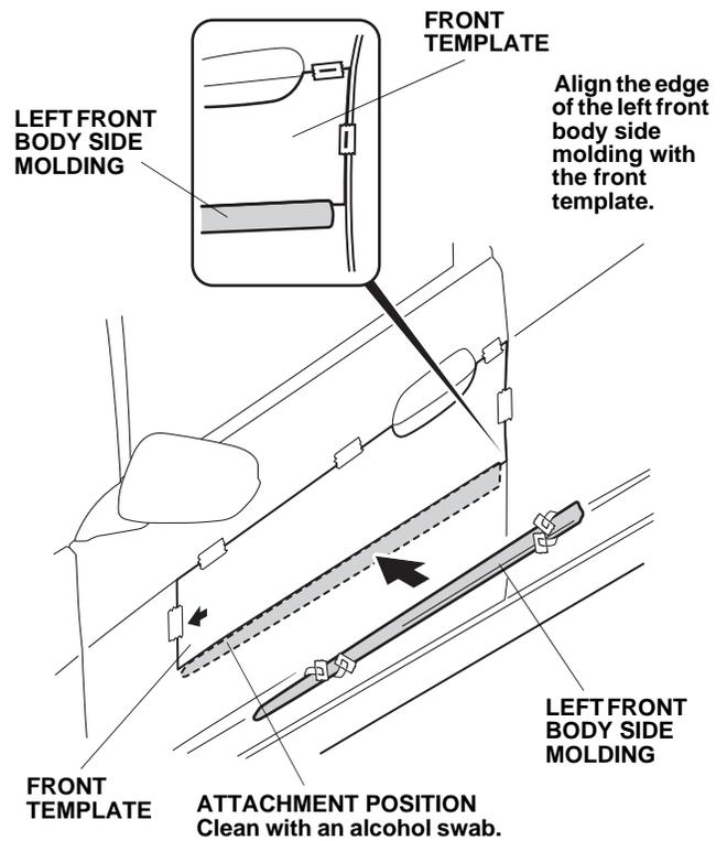
4. Align the left front body side molding with the front template and attach it to the driver's door. If the vehicle has door edge film installed, align the end with the door edge film.
