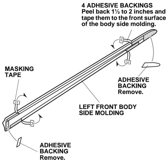
3. Clean the location where the left front body side molding will attach with one alcohol swab.
