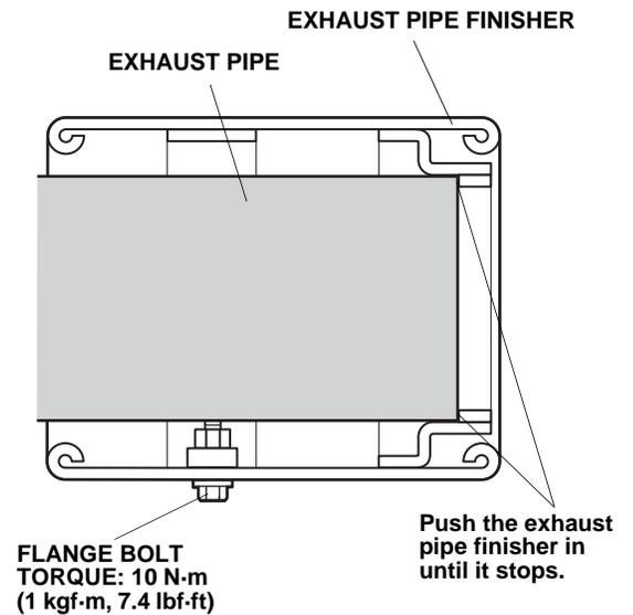
3. While pushing the exhaust pipe trim firmly against the pipe, torque the flange bolt to 10 N·m (7.5 lbf·ft).
