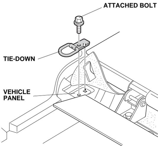
6. Repeat steps 2 through 5 to install a tie-down on the right side of the vehicle.
