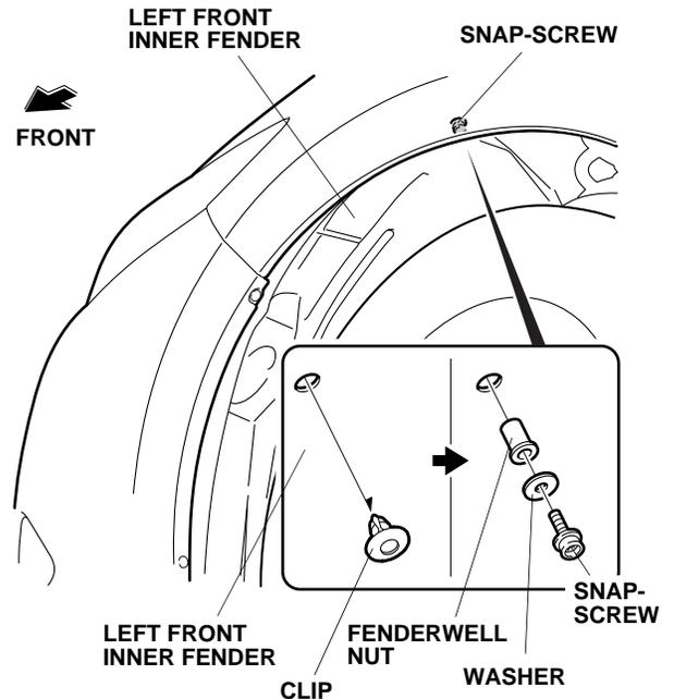
4. Attach one fenderwell nut into the left front inner fender.
