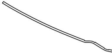
Seam sealant cutting tool
