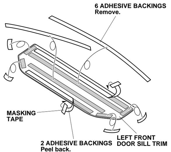
8. Remove the remaining adhesive backings.
