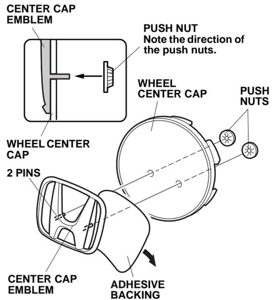
2. Remove the adhesive backing from the center cap emblem.
