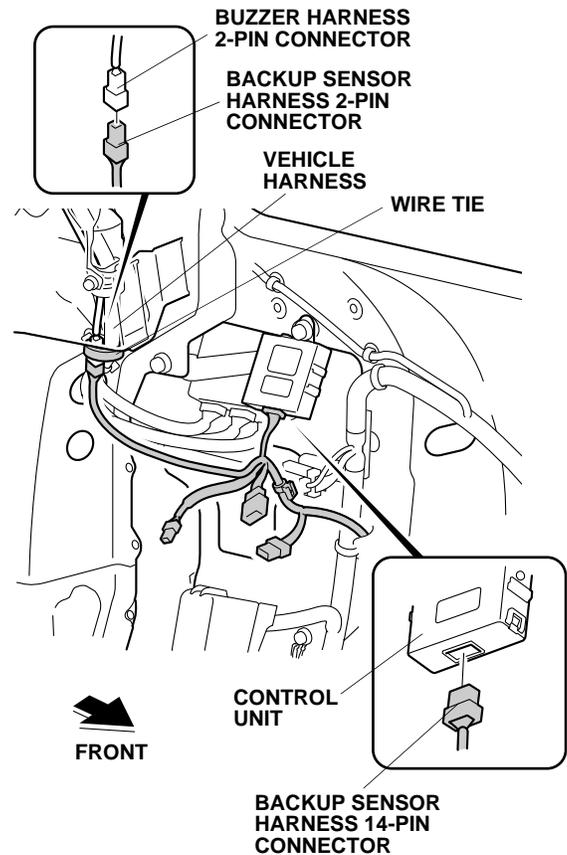
33. Plug the backup sensor harness 2-pin connector into the buzzer harness 2-pin connector.
