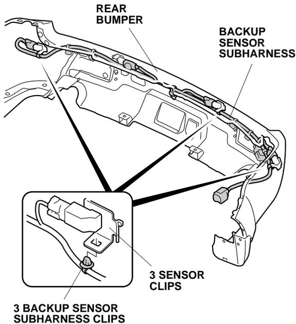
63. Secure the four backup sensor subharness clips to the four ribs on the rear bumper as shown.
