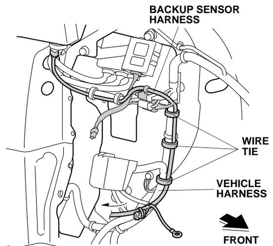
40. Remove the vehicle ground bolt from the vehicle ground terminal. Secure the backup sensor harness ground terminal to the vehicle ground terminal with the vehicle ground bolt just removed.
