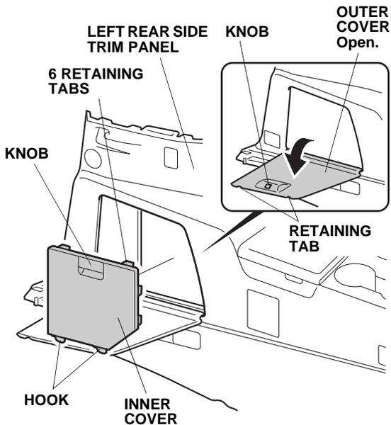
47. Pull the knob, and remove the inner cover from the left rear side trim panel (six retaining tabs and two hooks).
