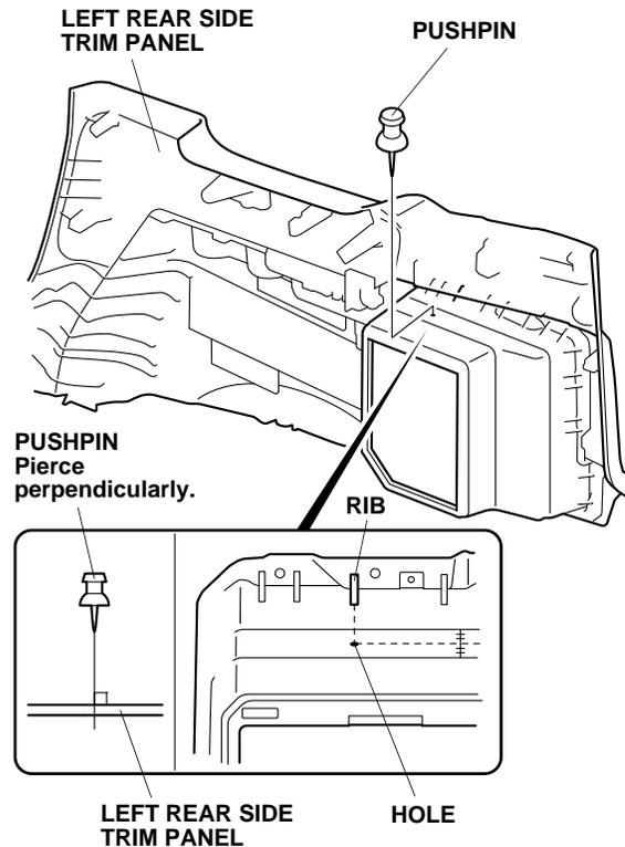
49. While wearing eye protection, drill a 3 mm hole at the pierced mark. Enlarge the 3 mm hole to 26 mm using a 26 mm hole saw.
