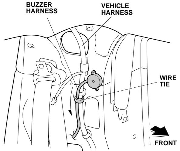
28. Continue routing the buzzer harness down along the vehicle harness, and secure it to the vehicle harness with three wire ties.
