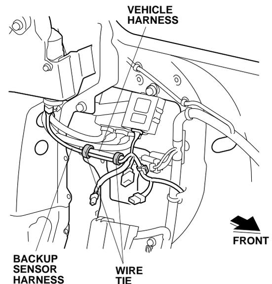
36. Unplug the vehicle 23-pin connector, and plug it into the backup sensor harness 23-pin connector. Plug the remaining backup sensor harness 23-pin connector into the vehicle 23-pin connector.
