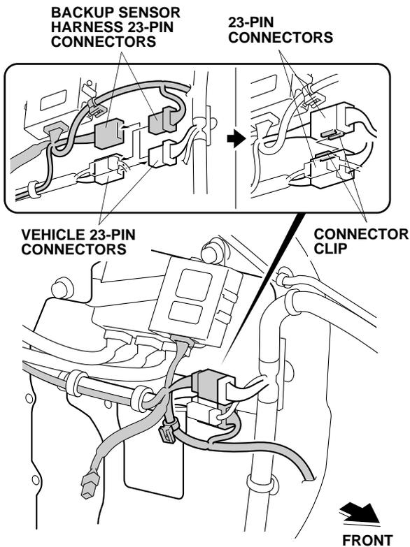
37. Attach the 23-pin connectors together using the connector clip.
