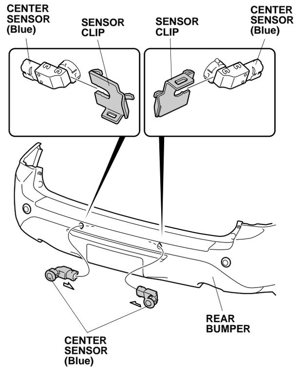
61. Plug the four backup sensor subharness 2-pin connectors into the four sensors.
