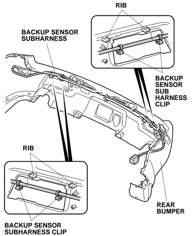
64. Secure the clip on the backup sensor subharness to the hole on the rear bumper as shown.
