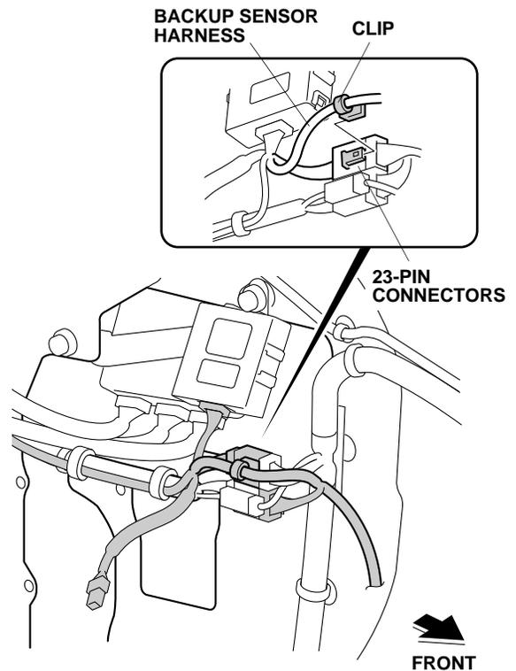
39. Route the backup sensor harness along the vehicle harness, and secure it to the vehicle harness with three wire ties.
