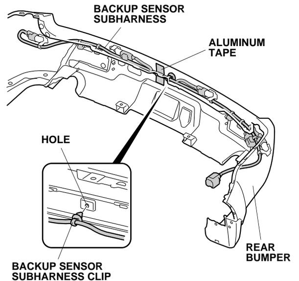
65. Using isopropyl alcohol on a shop towel, clean the rear bumper where the aluminum tape will attach. Secure the backup sensor subharness to the rear bumper with one aluminum tape.
