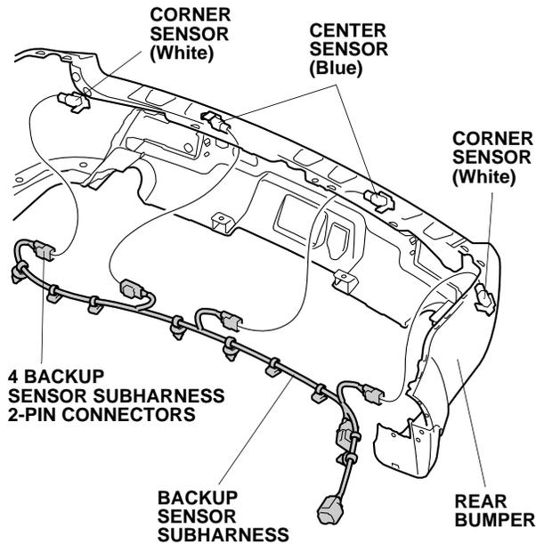
62. Secure the three backup sensor subharness clips to the three sensor clips as shown.
