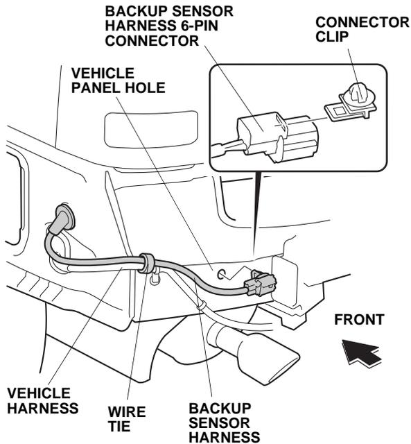
45. Secure the backup sensor harness to the vehicle harness with one wire tie.
