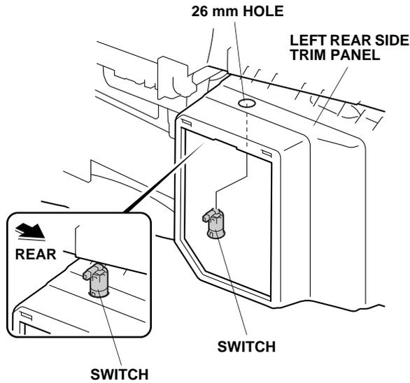
51. Using isopropyl alcohol on a shop towel, clean the switch bracket where the cushion tape will attach. Attach the remaining piece of cushion tape (from step 30) to the switch bracket as shown.
