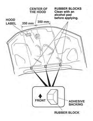
6. Remove the adhesive backings from the three rubber blocks and the hood label, and attach them to the hood at the measurements shown.
