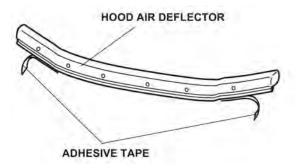
13. Align the holes on the hood air deflector with the brackets A, B, C. Install the hood air deflector with two screws, two collars, and four clips. Tighten the screws securely. Remove the adhesive backings.
