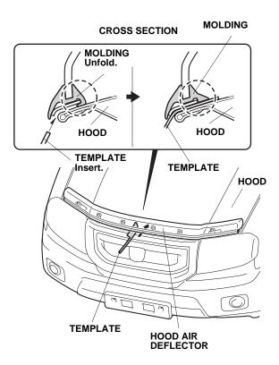
15. Open the hood. Tighten the four truss screws loosely installed in step 4.
