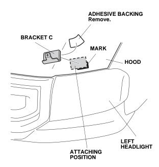
11. Turn the template over and repeat steps 7 through 10 to install the other bracket C on the right side of the hood.
