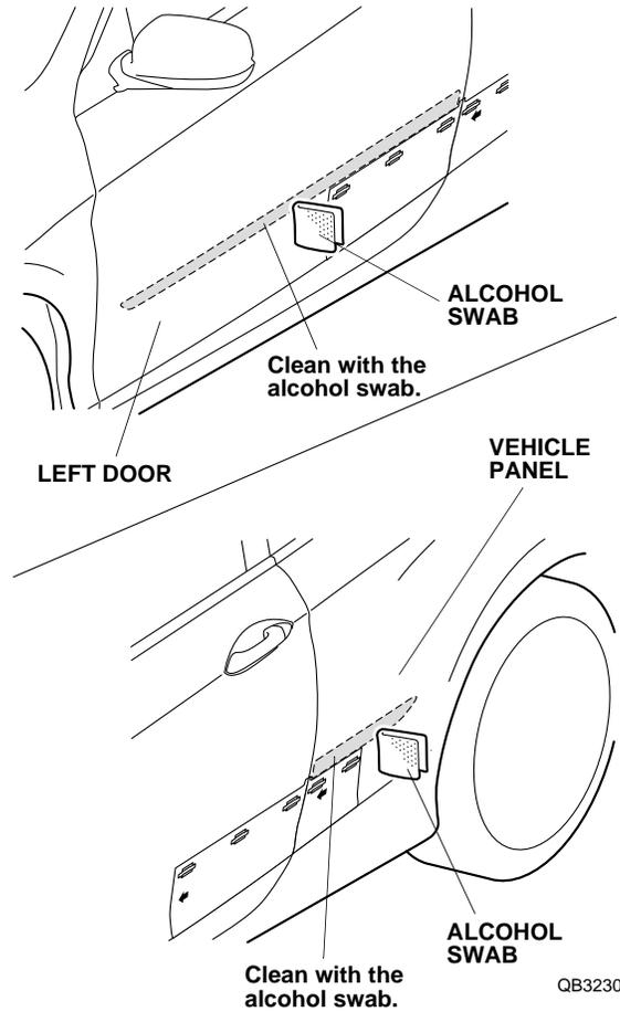
7. Peel back approximately 38 to 50 mm (1.5 to 2.0 in.) of adhesive backing from each adhesive strip, and tape the ends to the front surface of the body side molding. Remove the small end pieces of the adhesive backing.
