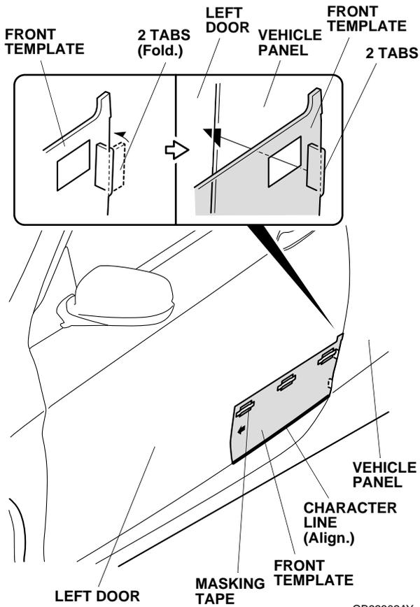
2. Insert the folded tabs of the front template into the opening between the left door and the vehicle panel. Align the template with the character line, and tape the template to the door with strips of masking tape.
