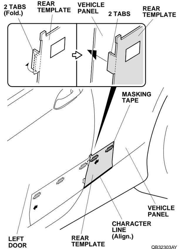
4. Insert the folded tabs of the rear template into the opening between the left door and the vehicle panel. Align the template with the character line, and tape the template to the door with strips of masking tape.
