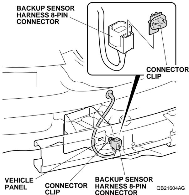
47. With the help of an assistant, bring the rear bumper next to the rear of the vehicle, plug the subharness 8-pin connector into the backup sensor harness 8-pin connector, and reinstall the rear bumper.
