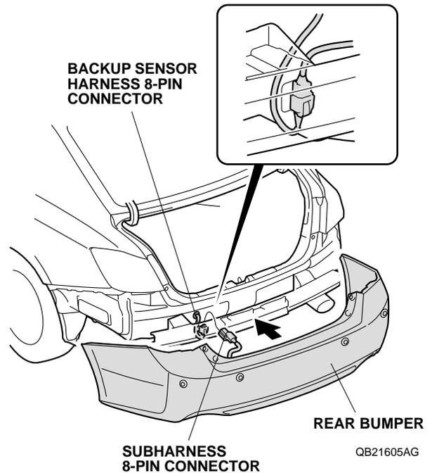
48. Check that all wire harnesses are routed properly and that all connectors are plugged in.
