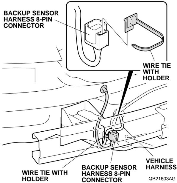
46. Install the connector clip to the backup sensor harness 8-pin connector, and secure it to the vehicle panel.
