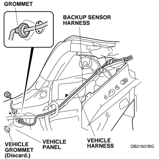
42. Locate and remove the vehicle grommet from the rear panel.
