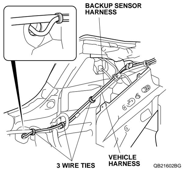
45. If equipped with vehicle harness, install the wire tie with holder to the backup sensor harness 8-pin connector, and secure it to the vehicle harness.
