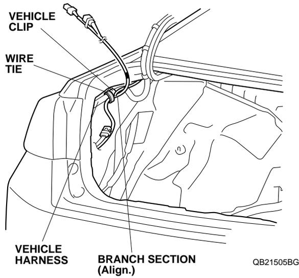
30. Align the green tape on the backup sensor harness with the vehicle clip, and secure the backup sensor harness to the vehicle harness with one wire tie as shown.
