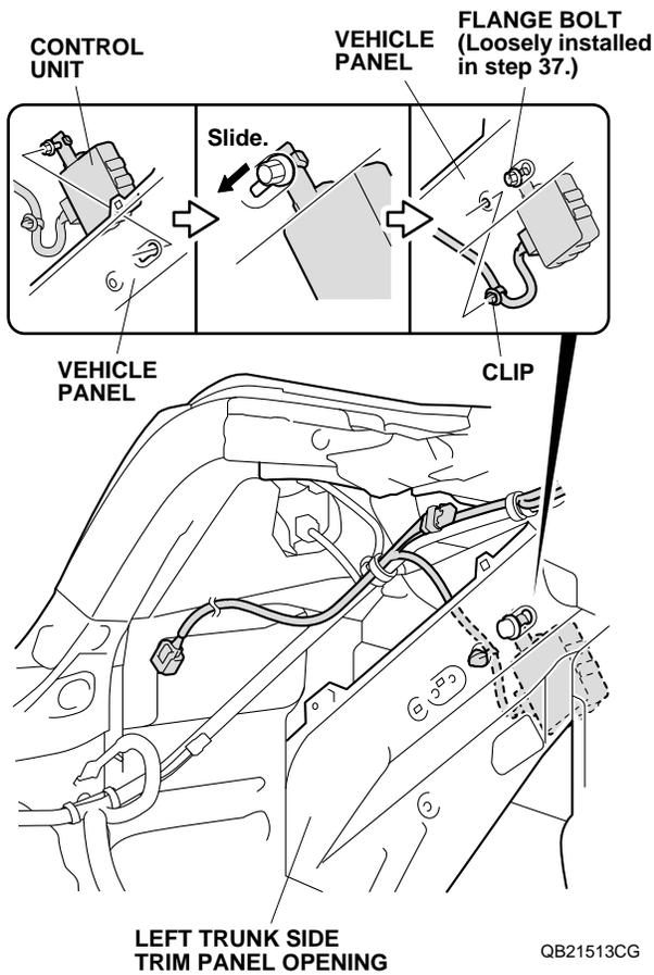
40. Secure the clip on the backup sensor harness to the vehicle panel.
