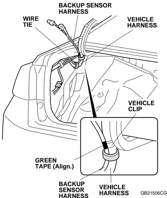
31. Secure the backup sensor harness to the vehicle harness with one wire tie.
