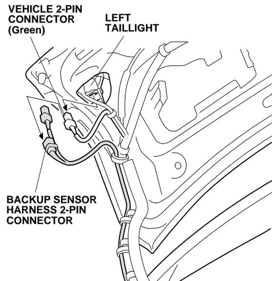
34. Plug the backup sensor harness 2-pin connector into the left taillight.
