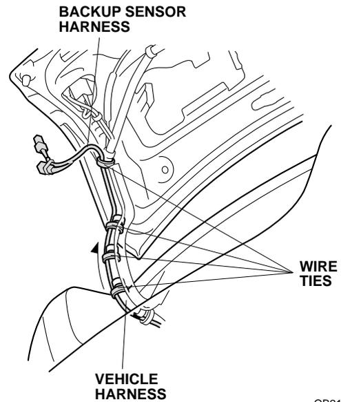
33. Unplug the vehicle 2-pin connector (Green) from the left taillight, and plug it to the backup sensor harness 2-pin connector.
