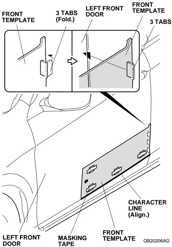
2. Insert the folded tabs of the front template into the opening between the front door and the B-pillar. Align the template with the character line, and tape the template to the door with strips of masking tape.
