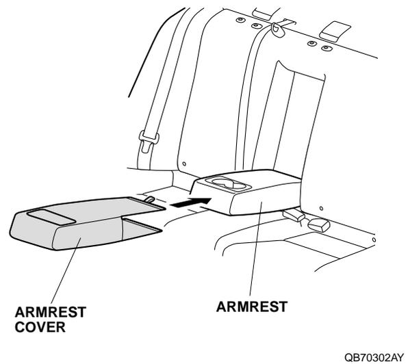
14. Raise the armrest. Pull out the armrest cover between the armrest and rear seat back, and secure the hook-and-loop fasteners on the armrest cover as shown.
