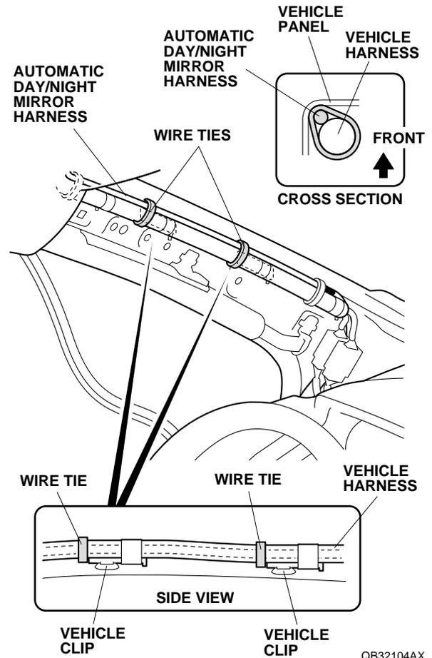
39. Check that all wire harnesses are routed properly and all connectors are plugged in.
