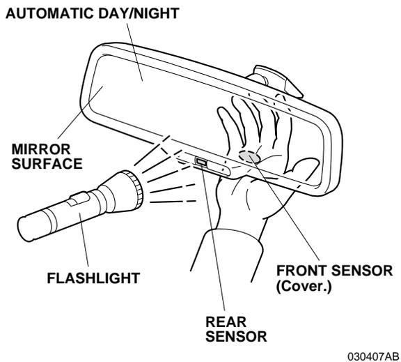
4. Step on the brake pedal, and move the select lever to the "R" position. Repeat step 3, and make sure the mirror surface does not dim.
