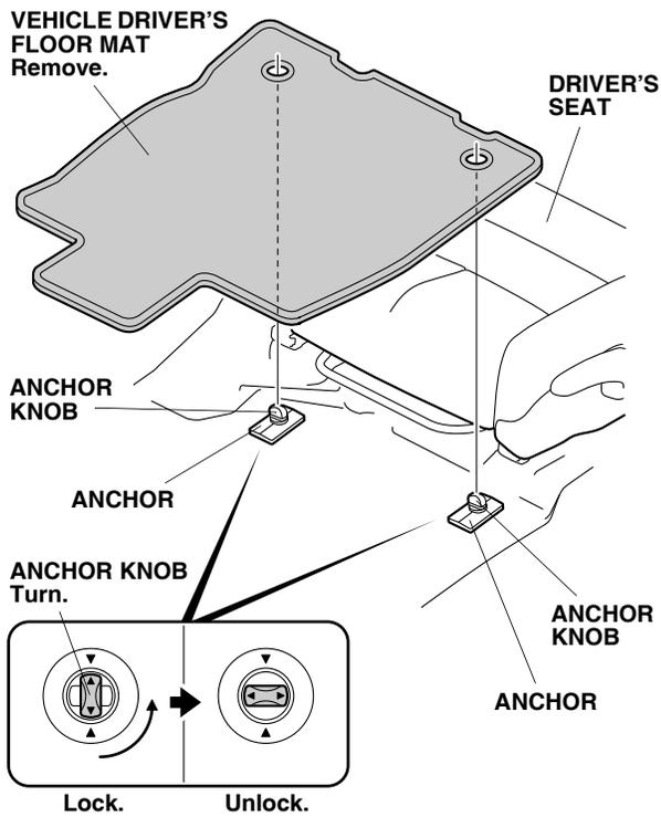
2. Install the rings in the driver's all-season floor mat over the anchors. Turn the knob on each anchor 90° to secure the driver's all-season floor mat.
