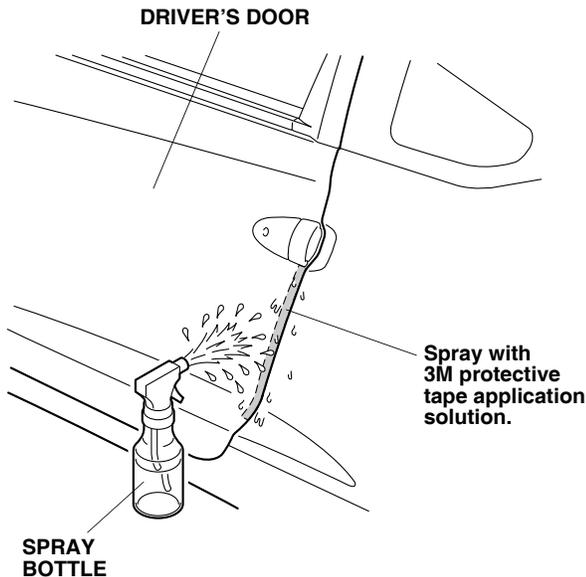
3. Open the driver's door. Peel back about 50 mm of the adhesive backing from the left door edge film. Align the v-notch on the left door edge film to the driver's door as shown.
