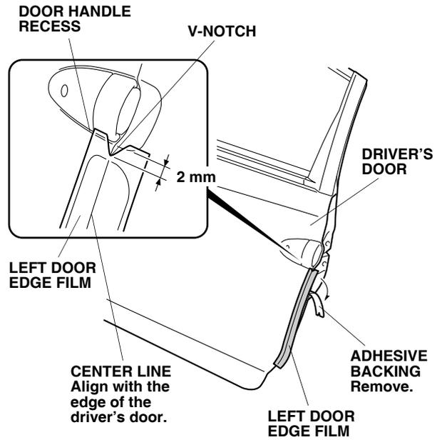
4. Align the center line on the left door edge film to the edge of the driver's door. While applying light pressure, carefully remove the adhesive backing, and attach the left door edge film to the driver's door.
