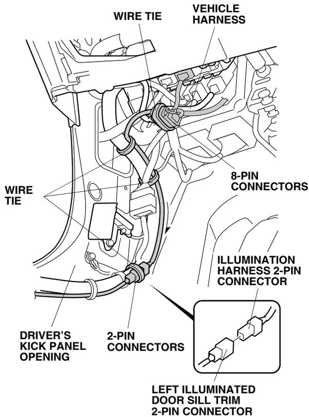
42. Secure the 8-pin connectors to the vehicle harness with one wire tie.
