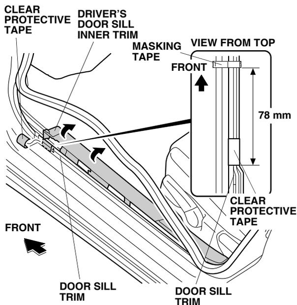
21. Using isopropyl alcohol on a shop towel, thoroughly clean the body where the clear protective tape will attach.
