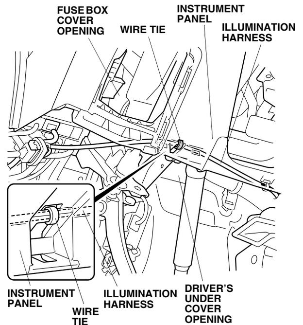
47. Route the illumination harness to the passenger's side of the vehicle as shown.
