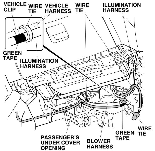
50. Secure the illumination harness to the vehicle clip with one wire tie at the green tape. Secure the illumination harness to the blower harness with one wire tie.
