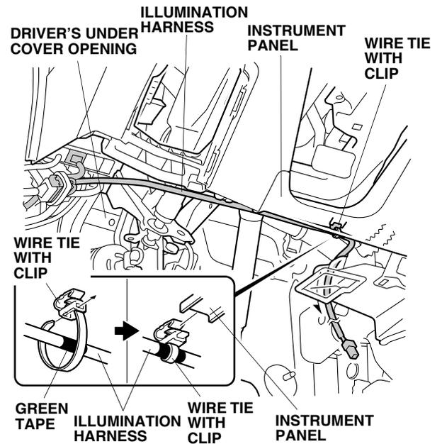
45. Attach one wire tie with clip to the illumination harness at the green tape. Clip it to the instrument panel.
