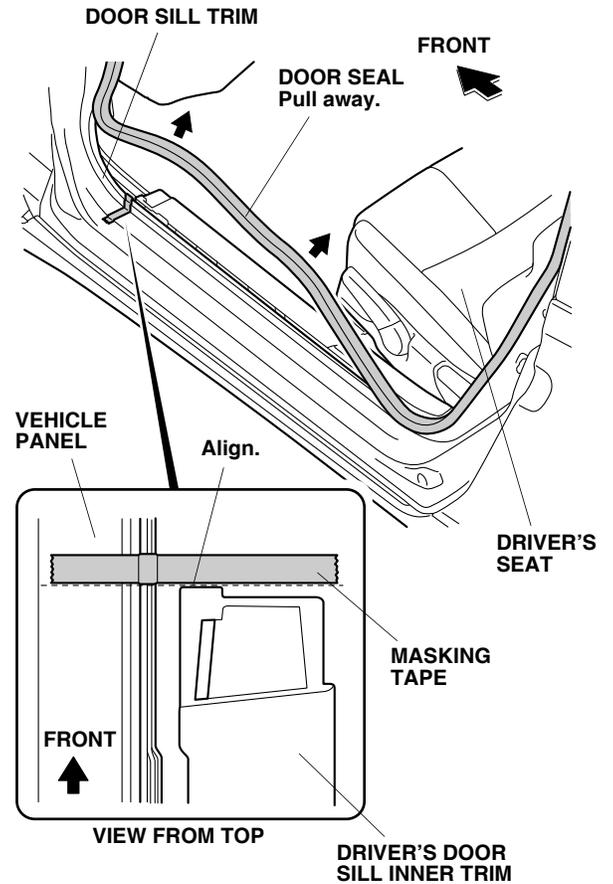
10. Attach a piece of masking tape to the vehicle panel. Align it with the front edge of the driver's door sill inner trim.
