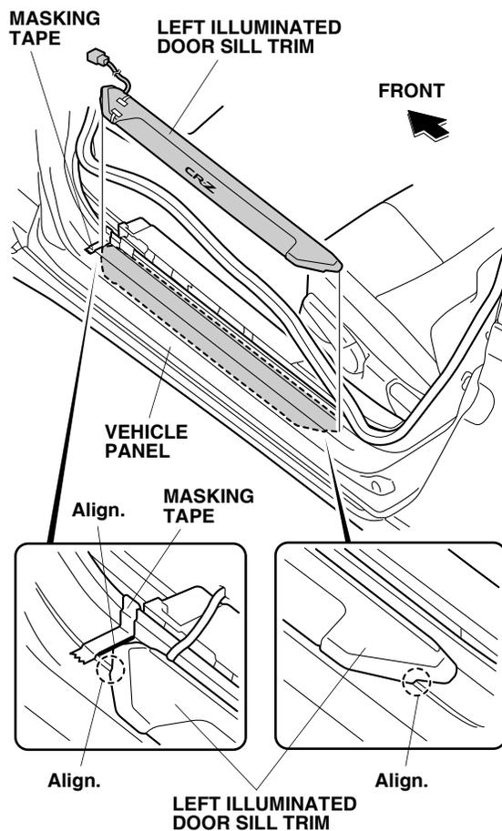
26. While applying light pressure against the left illuminated door sill trim, carefully remove the adhesive backings.
