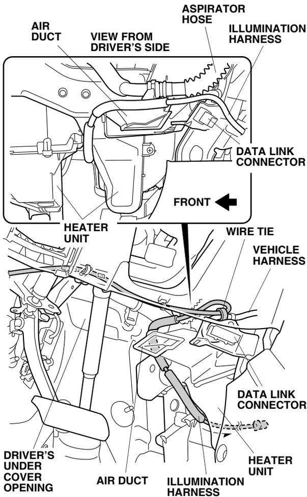
48. Secure the illumination harness to the vehicle harness with one wire tie.
