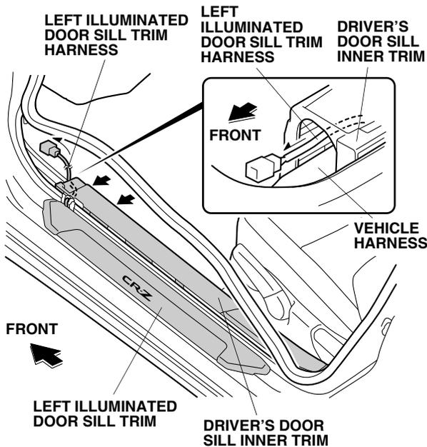
33. Reinstall the front of the driver's door sill inner trim and the door seal.
