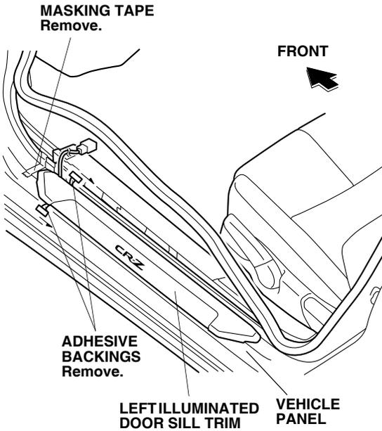
27. Using the palm of your hand, firmly press the left illuminated door sill trim against the vehicle panel.
