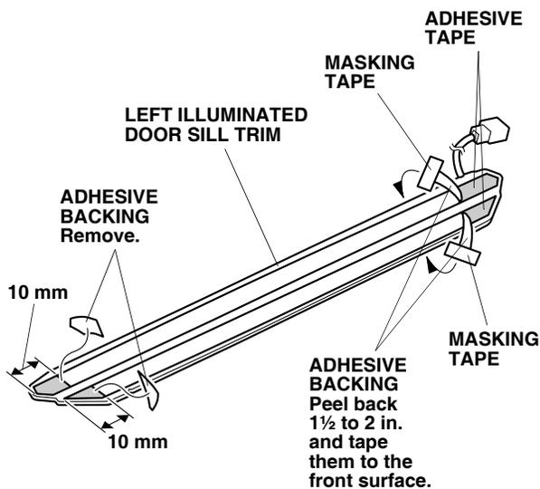
24. Using the alcohol swab, thoroughly clean the area where the left illuminated door sill trim will attach.
