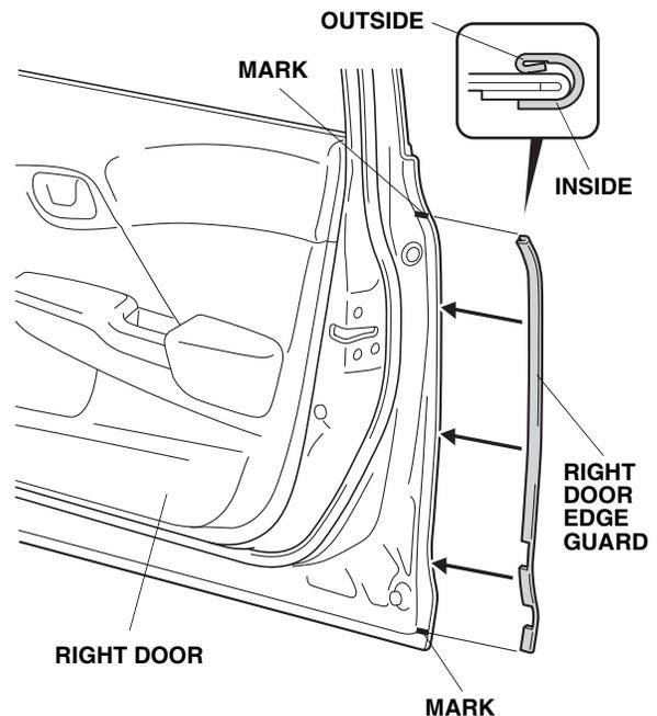
7. Starting at the character line, gently tap the right door edge guard into position with a series of light taps using a rubber mallet, then work up and down. Make sure the position of the right door edge guard is correct. Once in place, do not remove, reposition, or reinstall the right door edge guard or it will not hold securely.
